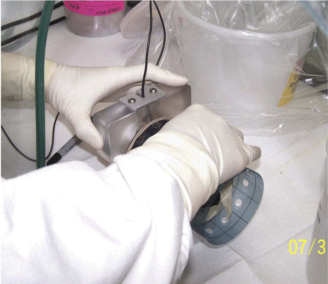
Figure 6. Photograph of Acquiring Thickness Measurements Using an Ultrasonic Testing Transducer.
