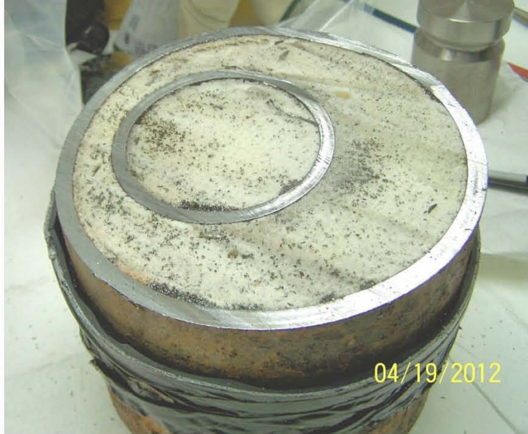
Figure 1. Photograph of the SN-278 Pipe-in-Pipe Section during Sample Unpacking.
