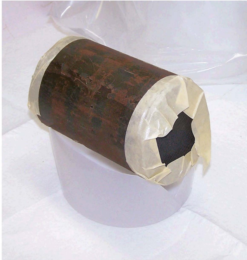
Figure 4. Photograph of SN-285 Pipe Section after the Final Cleaning Step.
