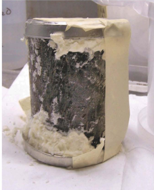
Figure 2. Photograph of the SN-278 Primary Pipe after Removal from the Pipe-in-Pipe Assembly.
