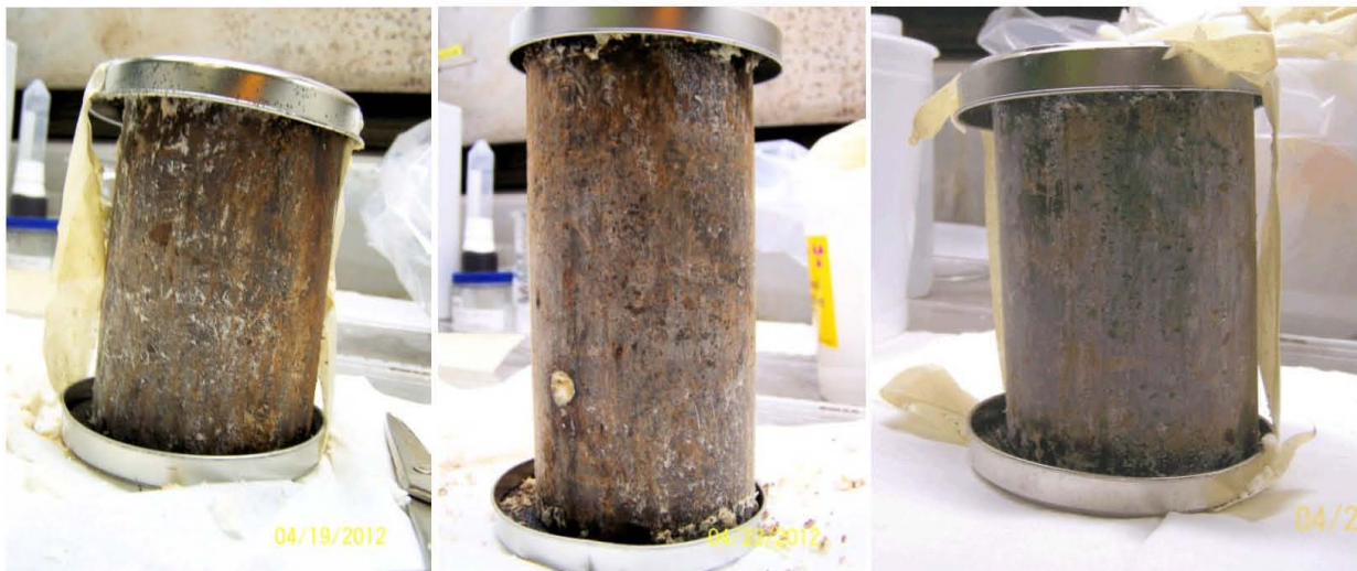
Figure 3. Photographs of the Cleaned Primary Pipes for Pipe Sections SN-285, SN-286, and SN-278.
