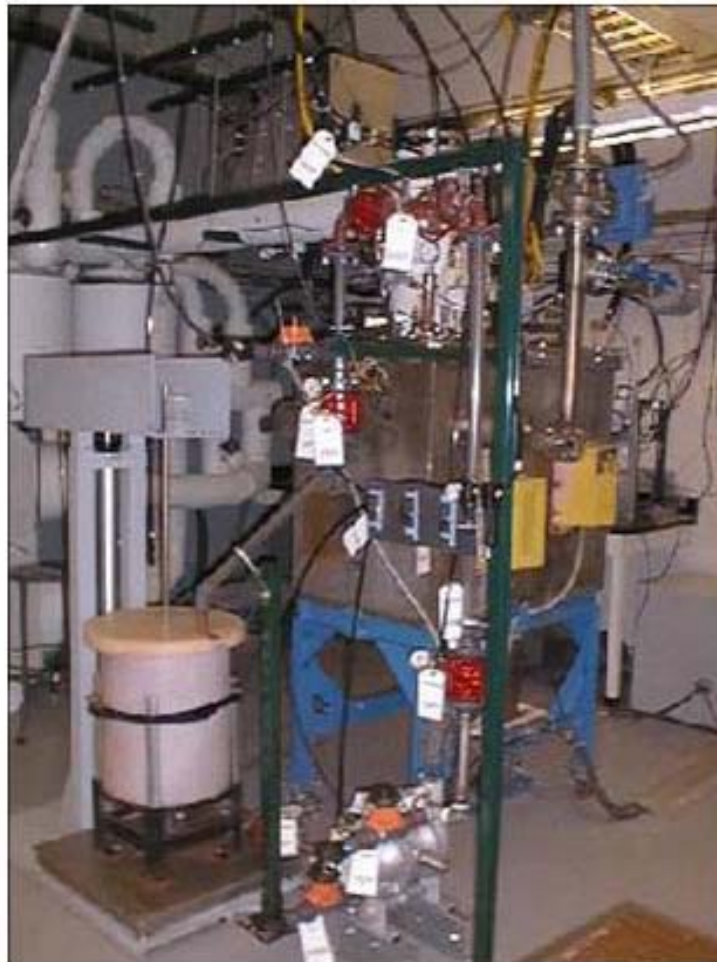
Figure 1.1. DML0 melter and feed tank; off-gas system is in the background to the left.
