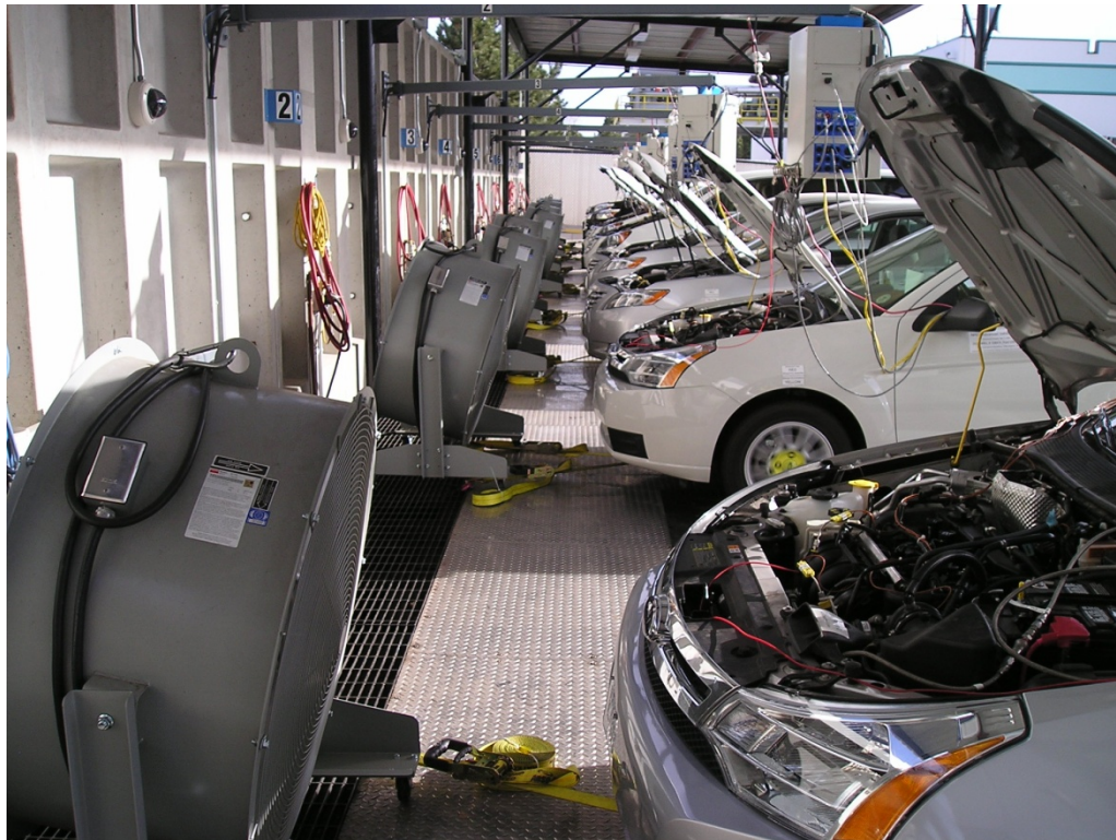
Figure 1. Test Vehicles Operating on the Mileage Accumulation Dynamometers Photos by SGS Environmental Testing Corporation
