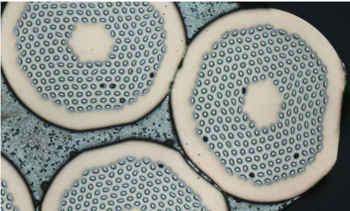
Figure 33. Close-up picture of the cable cross-section with PF of 82.8%
