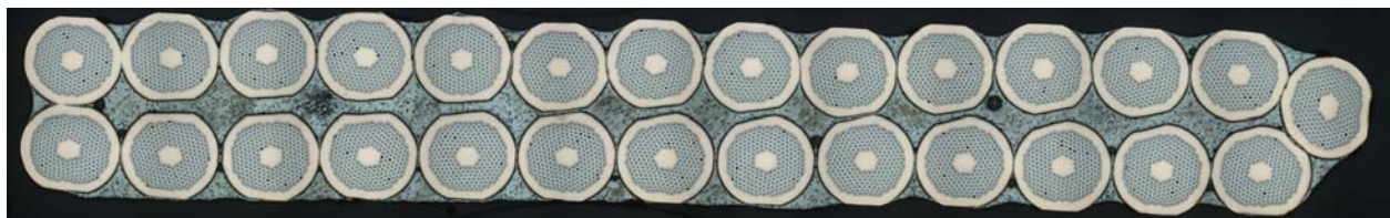
Figure 30. Cable cross-section with PF of 82.8%
