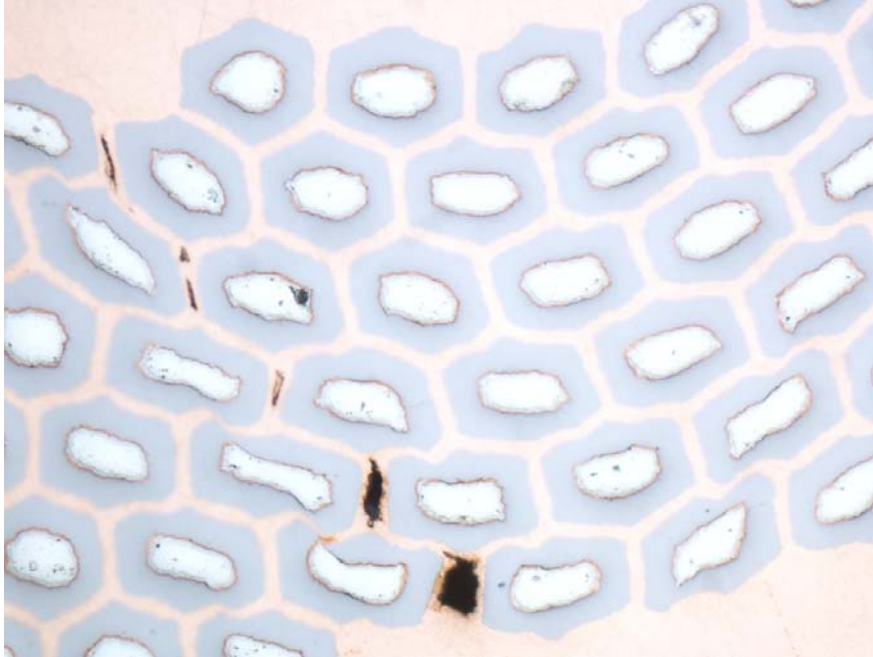
Figure 22. Cracked Copper between subelements.
