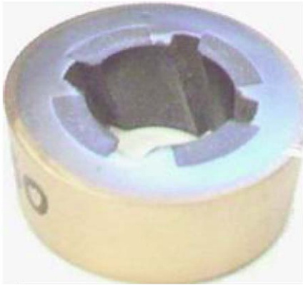
Figure 11. The skew of the magnetic poles is created during powder filling. The 1 mm thick Neo magnet and composite iron were co-filled and compacted together.
