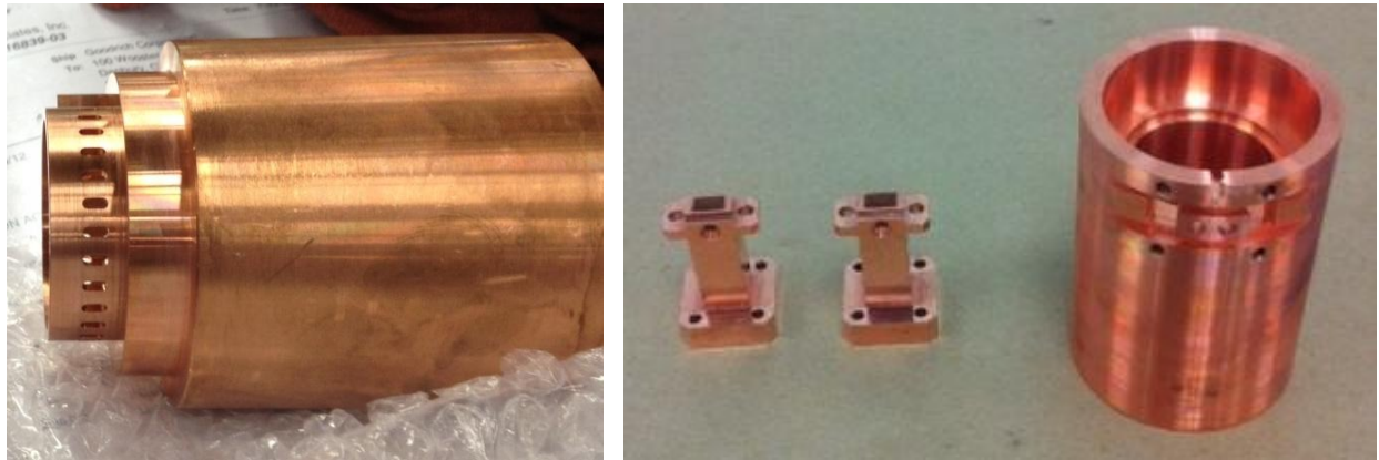
Figure 33. Parts for cold test version of output cavity.
