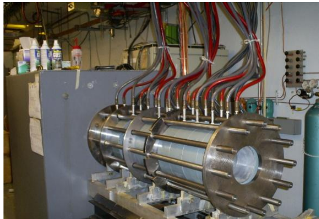
Figure 26. Solenoid magnet assembled at test, with gun tank seen at left.
