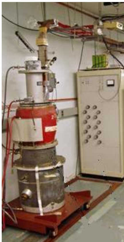
Figure 23. XK-5 S-band klystron. Modulator for electron gun described In the next paragraph is seen at the right-hand side of the photo.
