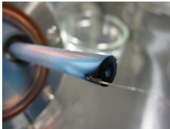
Figure 18: Tungsten oxide formed in 1350 torr of static xenon in a 0.58 L volume with 100 ppb oxygen
