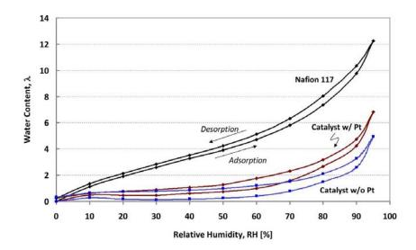
Figure 2. Water content as a function of humidity for bulk Nafion 117, catalyst-layer with 20wt% Pt/C and 5:2 Pt/C:Nafion, and catalyst layer with 2:1 C:Nafion.
