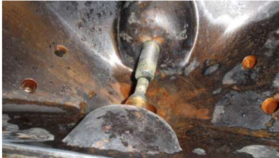
Figure 5.1.13. All-steel negative electrode with large cross-section installed in chamber.
