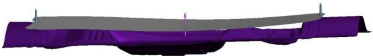
Figure 7.3. Blank location after gravity phase. 2 pins control the blank location.
