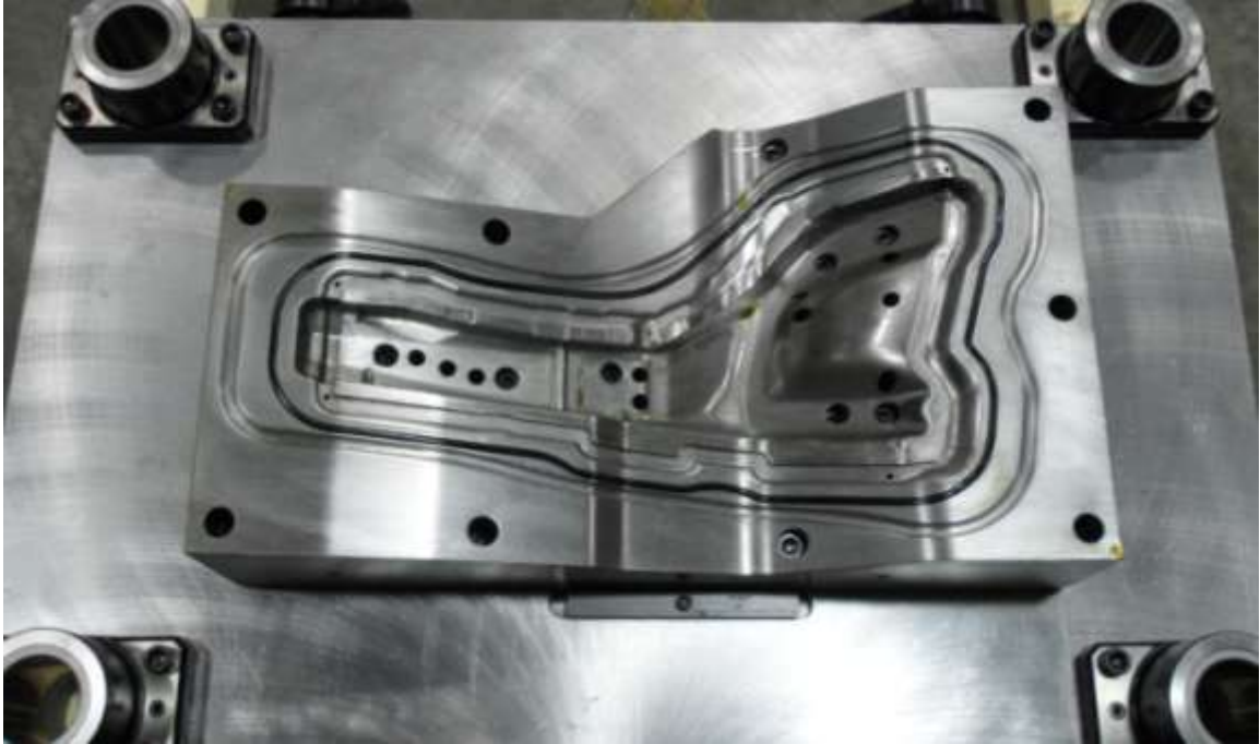
Figure 6.1.10. Upper half of EH trimming tool, including trim blades.
