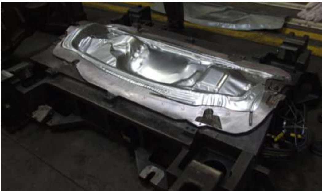
Figure 7.18. Preformed blank positioned inside the lower die during measurements of the material inflow into the die cavity.
