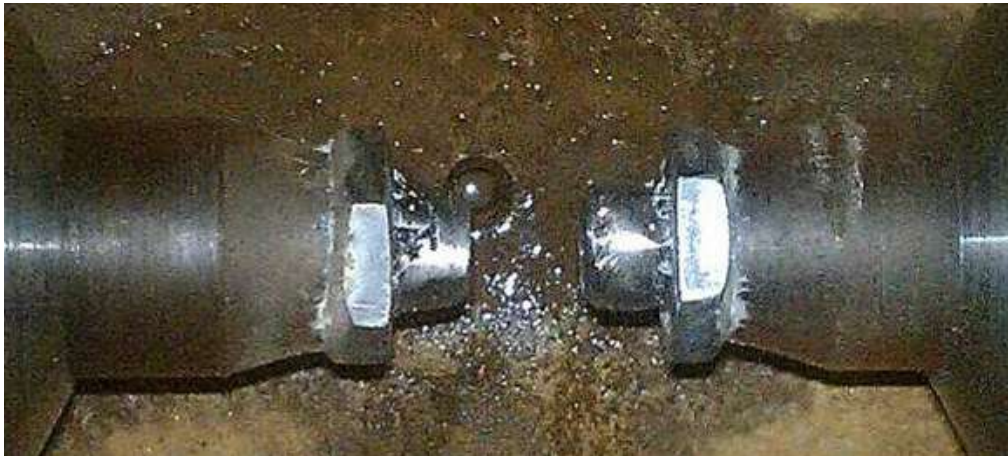
Figure 2-18. Half nuts welded to conical insulation tip electrodes, as seen before testing. Note that the welds were placed on the electrode tip side (not the insulation side) and some damage occurred to the insulation as a result of welding.
