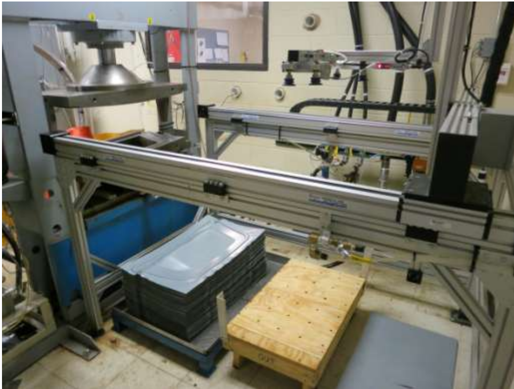
Figure 3.3.2. Material Handling Gantry. Input blanks are placed on wood pallet and finished parts are placed on the stack in the pan.
