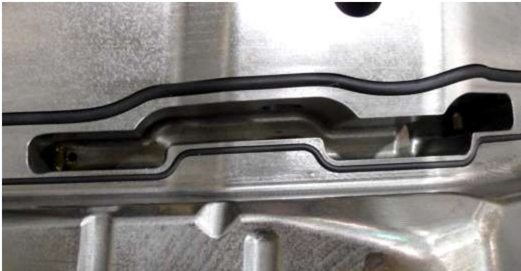
Figure 6.1.11. Close-up view of one of the fluid sub-channels. The lower edge in the image - the edge closer to the smaller seal groove - corresponds to the trim line of the panel.
