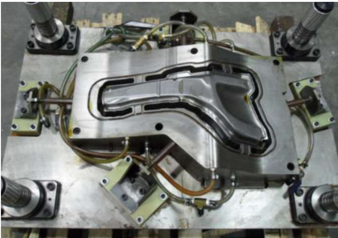
Figure 6.1.9. EH trimming tool, lower half, including four fluid sub-channels.
