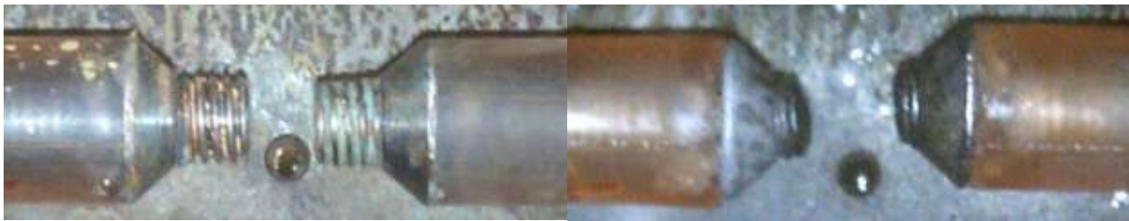
Figure 2-20. Results of electrodes test with machined insulation protection tip. Weld placed behind protector and insulation cast on after welding, as seen at left. Photo at right shows the electrodes in the chamber suspended after 1000 pulses were applied.
