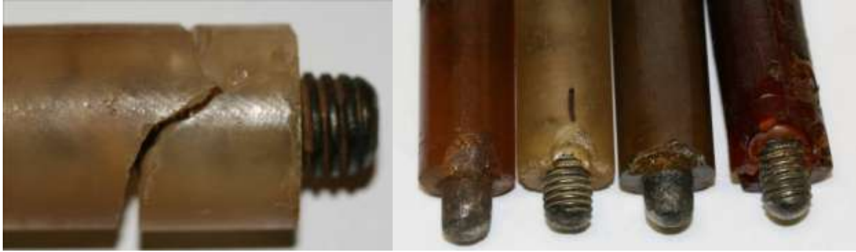
Figure 2-14. Typical (polyurethane) insulation damage observed on electrodes with square insulation profiles after 120 pulses. Note both chipping and separation of insulator from electrode shaft.
