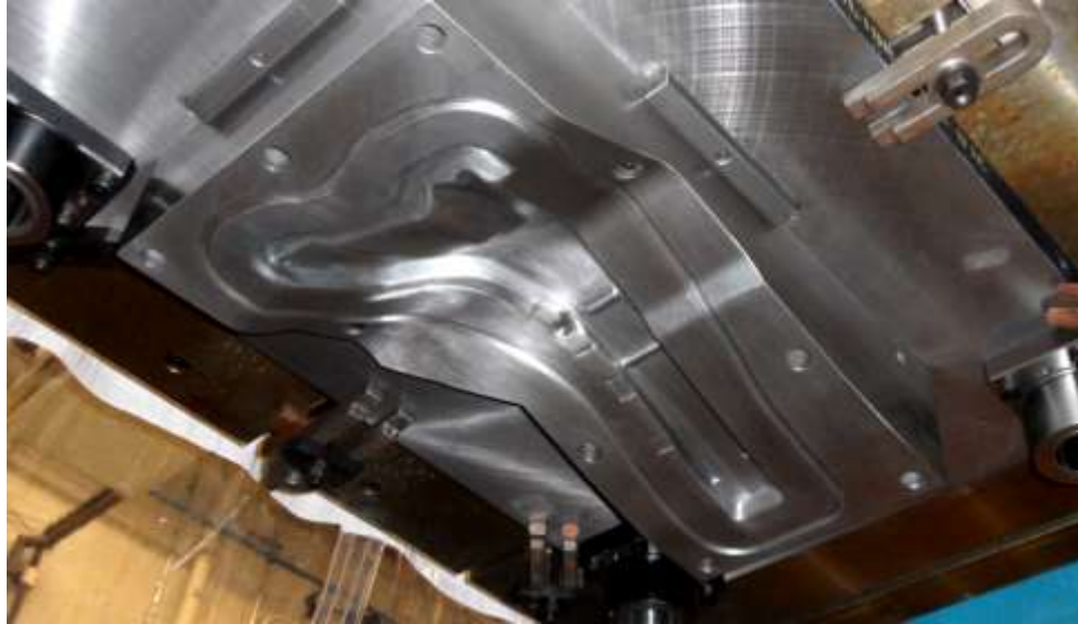
Figure 6.2.17. Overall view of the upper half of the EH calibration tool, which consists of a female die surface cut to the desired part geometry.
