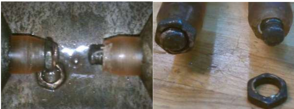
Figure 2-19. Results of test of electrodes with welded nuts as insulator protection – weld erosion and failure after 480 pulses. Both nuts were loose as significant damage occurred to threads after weld failure.
