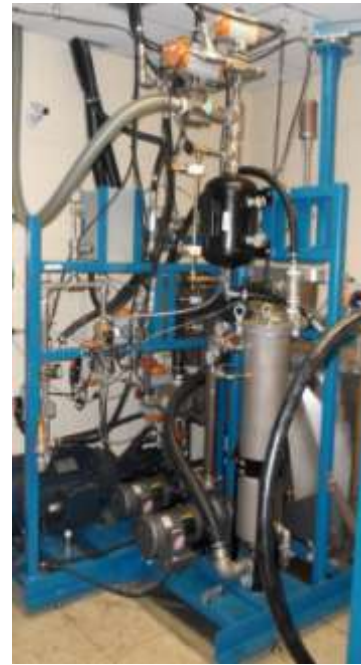
Figure 3.1.3. The two-skid, primary portion of the Fluid Handling System.
