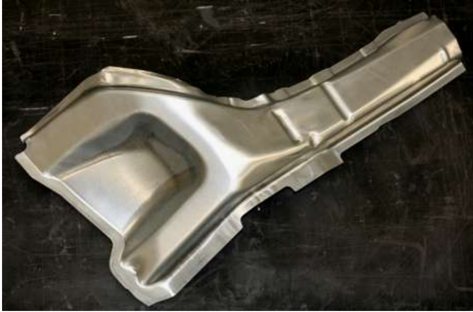
Figure 6.1.13. Front floor side inner panel, trimmed using EH trimming.
