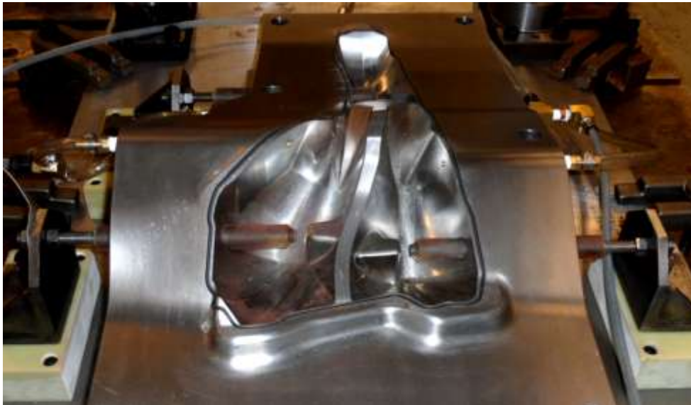
Figure 6.2.16. Close-up view of the two sub-chambers near the back end of the EH calibration tool, showing the position of the energized electrodes and the ground electrodes.
