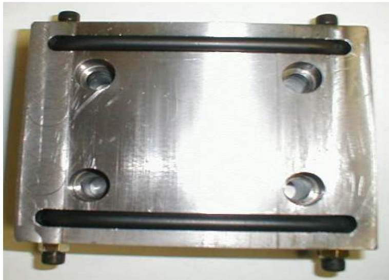
Figure 3.2-5. Groove plate carrying two rubber seals for wear testing.
