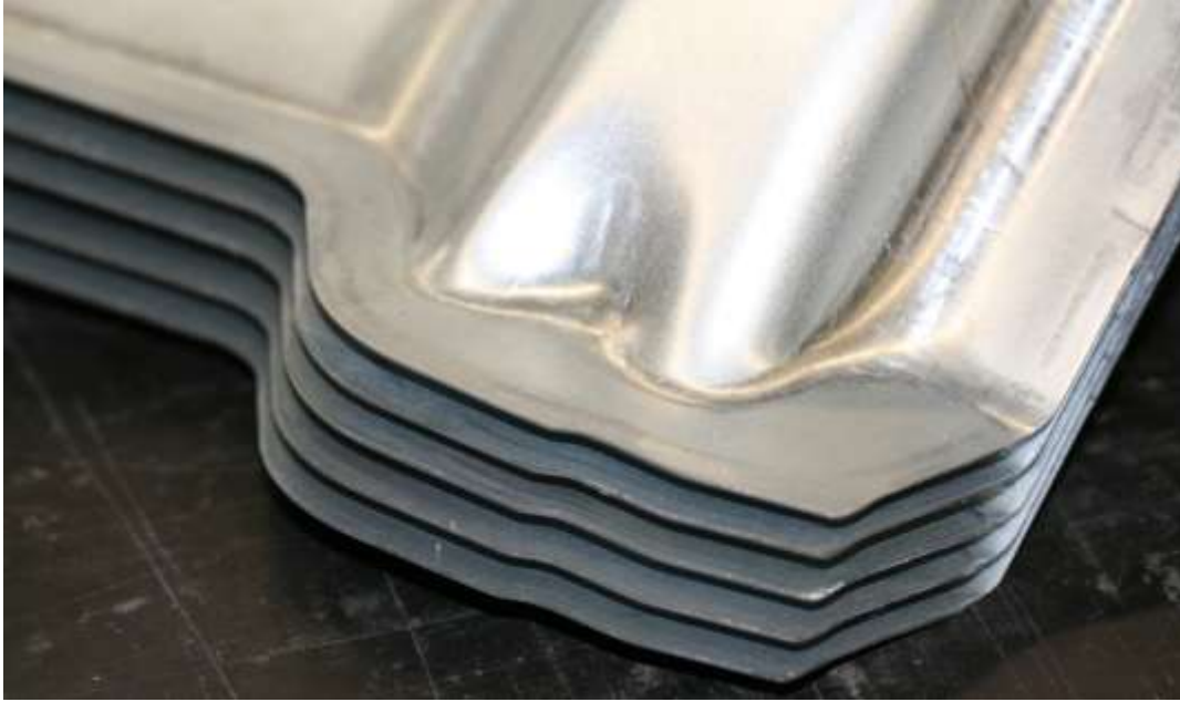
Figure 6.1.15. A stack of panels trimmed using EH trimming, revealing the absence of any burrs and a clean trim edge matching the fine details of the part geometry.
