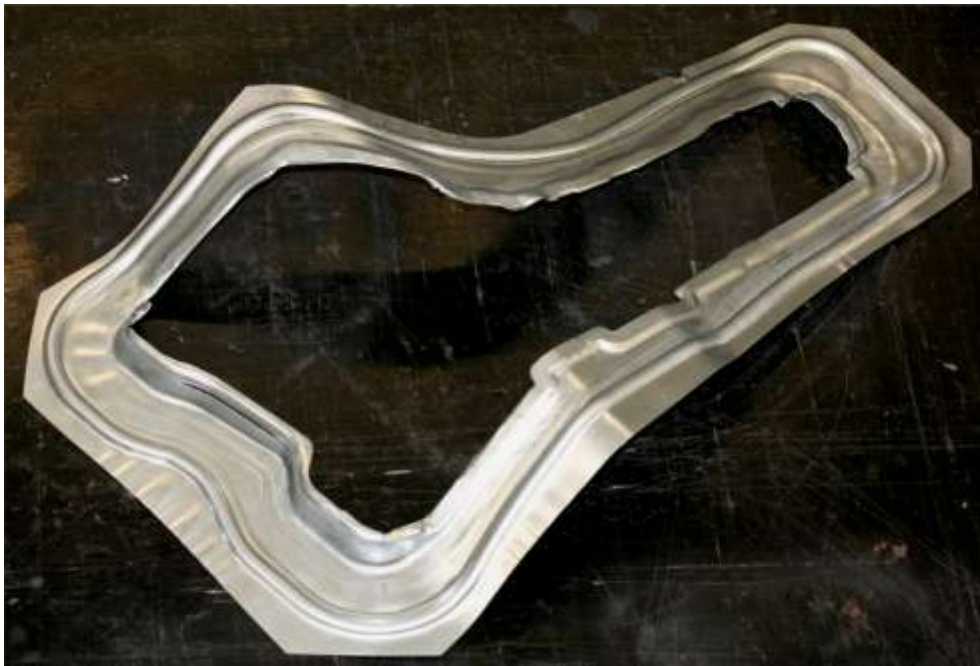
Figure 6.1.14. The offal resulting from EH trimming of the floor side inner panel.
