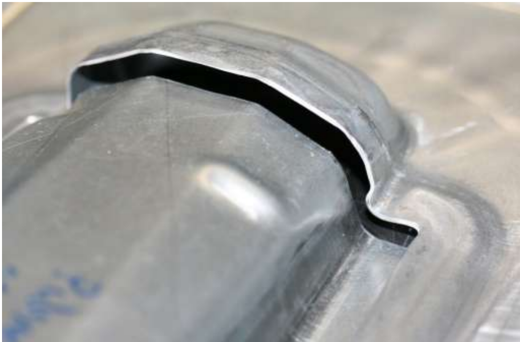
Figure 6.1.16. The front nose of the floor side inner panel partially trimmed using EH-trimming. The mechanism of EH-trimming can be seen in the photograph: the part-side of the metal is clamped in place, and the scrap-side of the metal is deformed upward and outward, against the sharp trim edge and away from the part-side.
