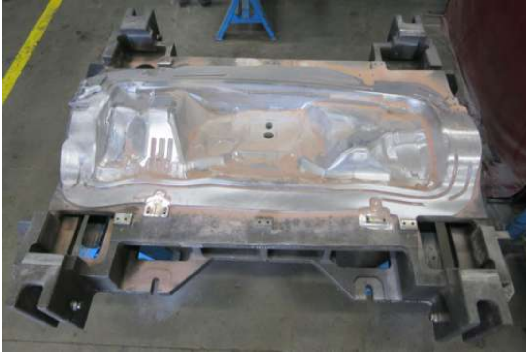
Figure 7.16. Assembled lower preforming die.
