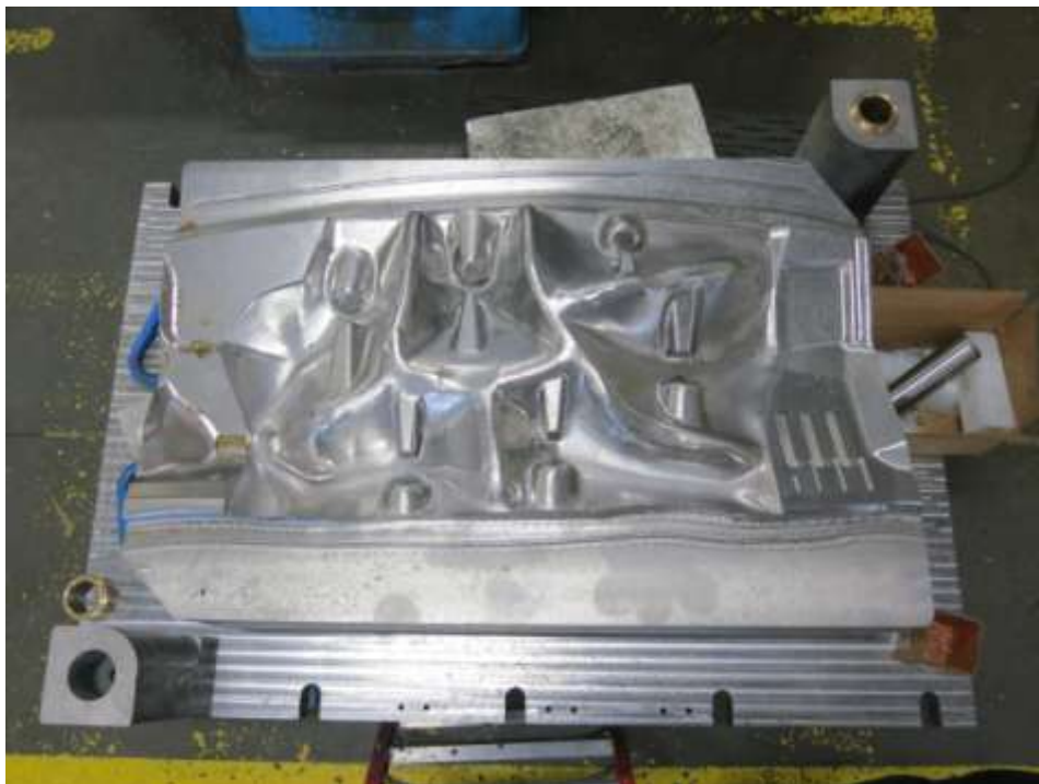
Figure 7.21. EHF chamber prior to the installation of electrodes.
