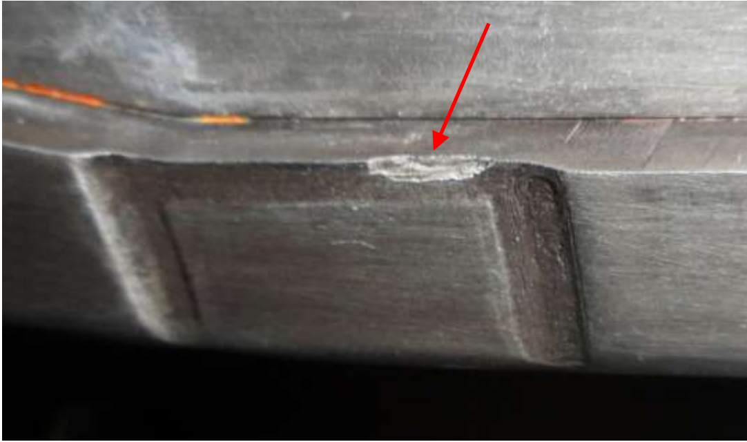
Figure 6.1.17. A small area of chipping on the sharp trim edge in the large EH trim tool.
