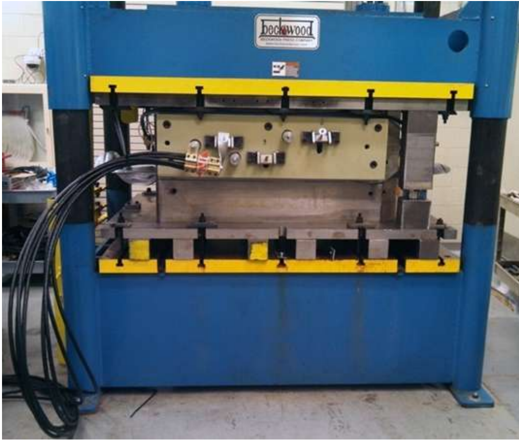
Figure 7.23. EHF tooling in closed position during the tryout process at the Ford Norwood lab.
