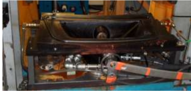
Figure 5.1.2. The new chamber optimized to decrease cycle time by reducing the volume from 19 to 11 liters and enlarged porting.
