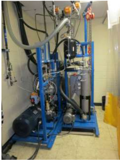
Figure 3.1.3. The two-skid, primary portion of the Fluid Handling System.
