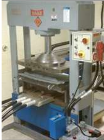
Figure 3.3.3. Original press now upgraded with new pump, manifold, and controls. See Figure 3.3.6 for a picture of upgraded press.
