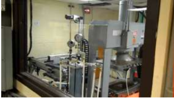
Step #1: Gantry retrieves part blank from stack
