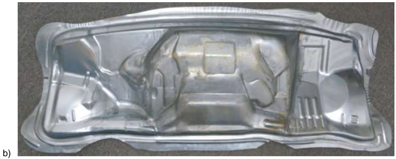
Figure 7.24. The fully formed dash panel (1.5 mm DP600) after EHF forming. a) Viewed from the EHF chamber side. b) Viewed from the die side.
