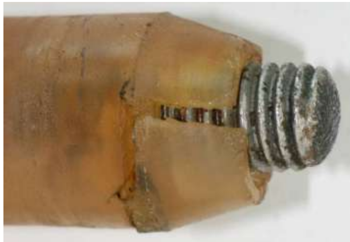
Figure 2-15. Typical (polyurethane) insulation damage observed on polyurethane electrodes with conical insulation profiles. After 120 pulses no significant damage was noted. This failure occurred after 650 pulses were applied. Note relative lack of insulation chipping. Failure observed in both electrodes includes circumferential cracking of insulation just behind the conical region, separation of insulator from electrode shaft, and final longitudinal failure of insulation.
