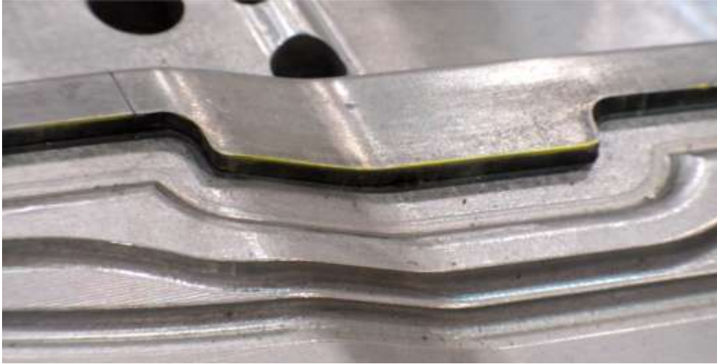
Figure 6.1.12. Close-up view of the edge of the trim blade (shown protruding above the offal guiding area or offal space). This region of the trim line corresponds to the central region of the fluid channel shown in Figure 6.1.11.
