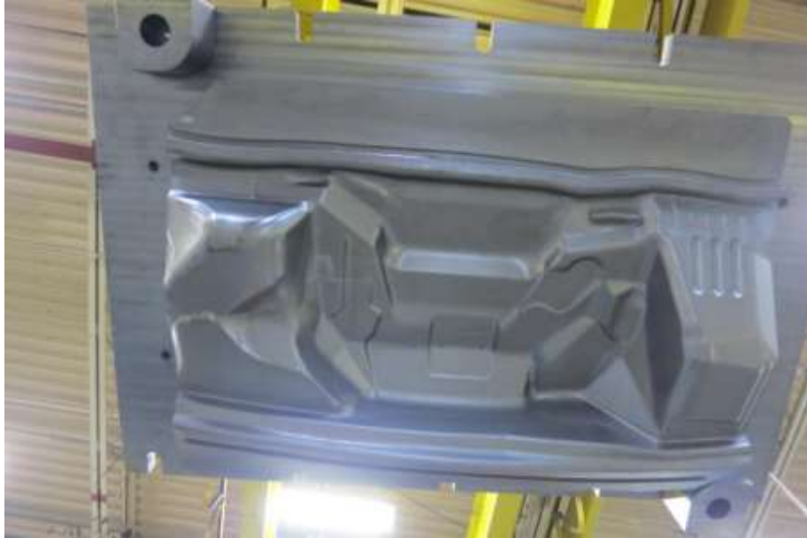
Figure 7.20. EHF die providing final shape forming.
