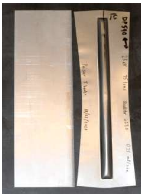
Figure 4.2.15. Photographs of blanks before and after forming. The draw-in length for each formed specimen was computed by subtracting the final width (measured at the middle of the blank) from the initial width.
