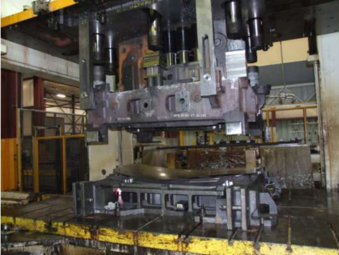
Figure 7.17. The assembled preforming die installed in a 3000 ton, double action hydraulic press at Amino NA during the tryout process.
