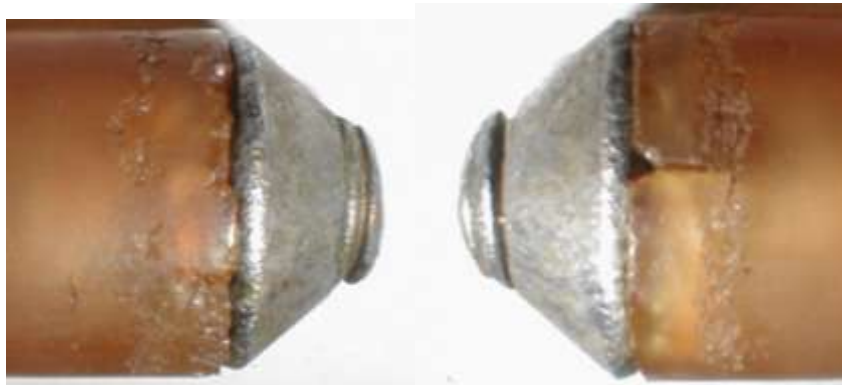
Figure 2-21. Detail of damage observed in test of machined and welded insulation electrode protection tip. Note general insulation erosion, chipping, and longitudinal crack formation.
