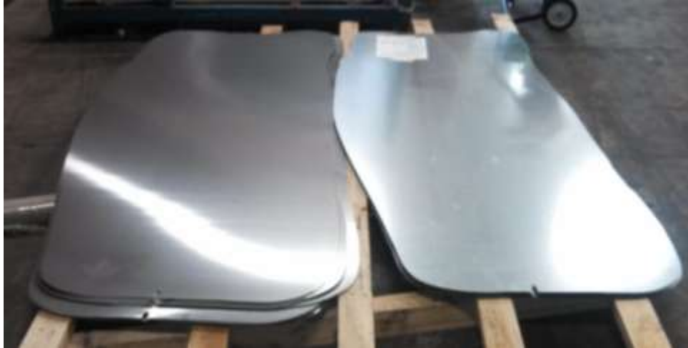
Figure 7.13. Individual flat blanks laser trimmed from 1.5 mm thick DP600 sheet.
