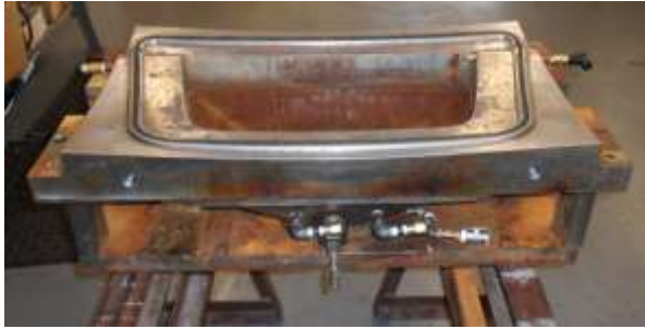
Figure 5.1.2. The new chamber optimized to decrease cycle time by reducing the volume from 19 to 11 liters and enlarged porting.
