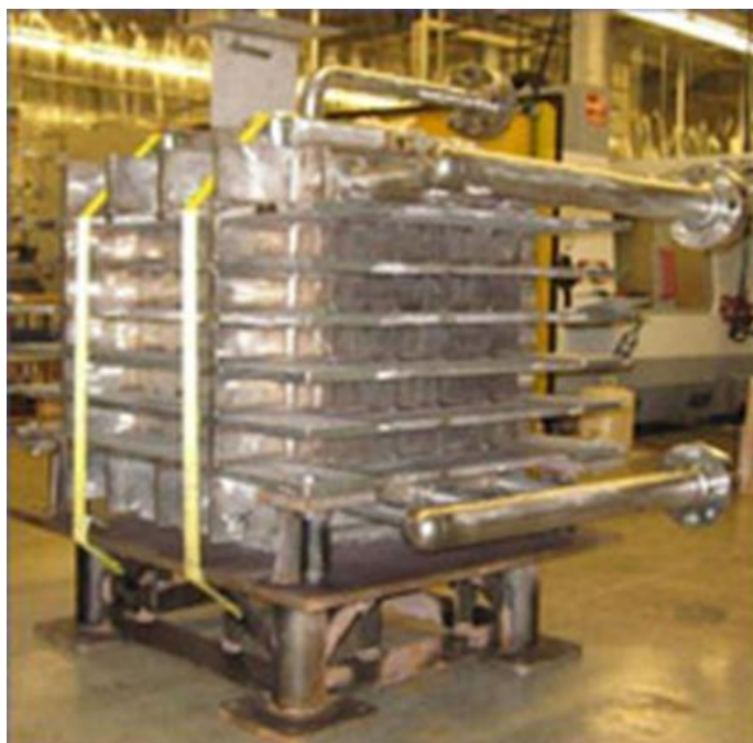
Figure 10: Velocys commercial Fischer-Tropsch Reactor
