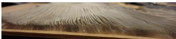
100 wire mesh, 30 FPI, 0.1" Fin height, 18" fin length
