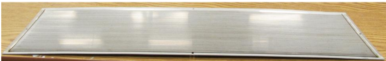
Figure 20: Laser welded assembly with minimal deformation produced by improved manufacturing
