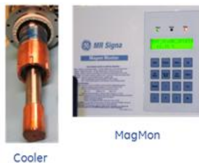
Figure 19 - Main components: cooler and MagMon (magnet monitoring system)
