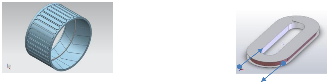
Figure 17 – (a) Aluminum 6061 coil former with machined race track coil pockets (36 pole design)
