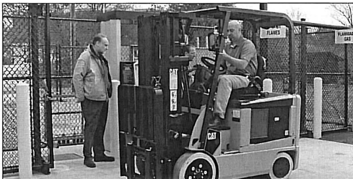
The USC-Columbia Fuel Cell Collaborative partnered with LiftOne and Hydrogenics to deploy two fuel cell powered forklifts in real-world operation in the region.
