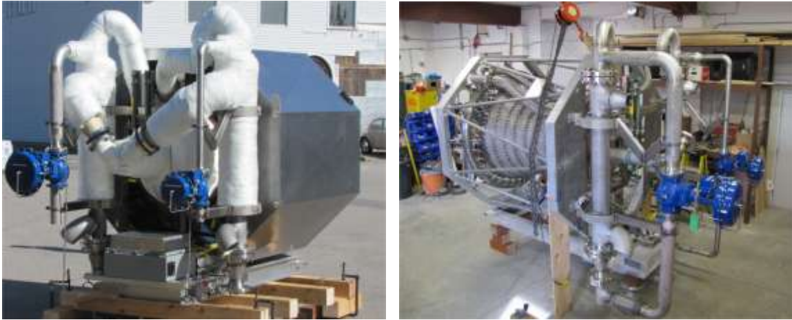
Figure 2.7 Photograph of solar receiver test rig during final assembly.
