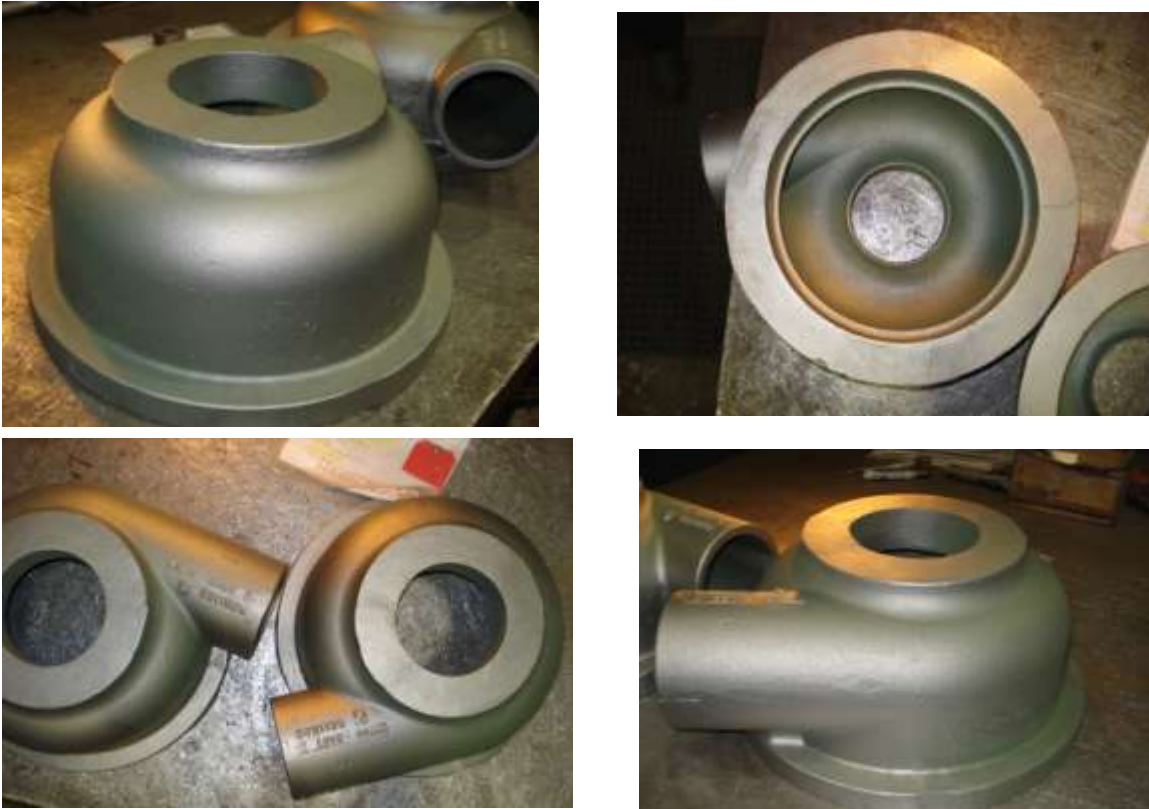
Figure 5 - SolarCAT Stage-3 turbine housing, case from Hastelloy-X. The diameter is about 10 inches.
