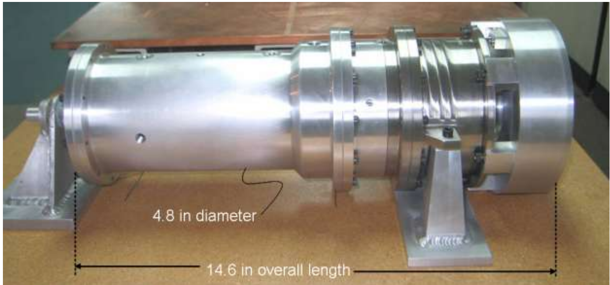
Figure 6. Assembled turbo-alternator simulator. This contains the alternator and complete bearing system. Over 100 hours of hot and cold rotor testing was performed, covering the entire speed map up to 120,000 RPM.
