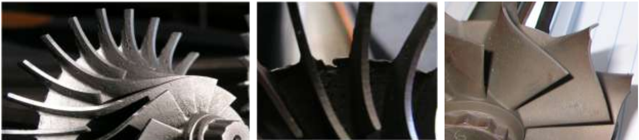
Figure 2.2 – Photos of the Stage 1 (left and center) and Stage 4 (right). Stage 1's narrow blades, poor surface finish, and poor casting quality are evident in the prototypes.
