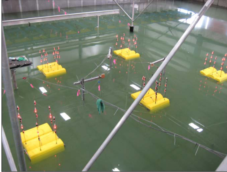
Figure 15: The photo shows the WEC array experiment for the 5 WEC case conducted in the O.H. Hinsdale Tsunami Wave Basin at Oregon State University [1].
