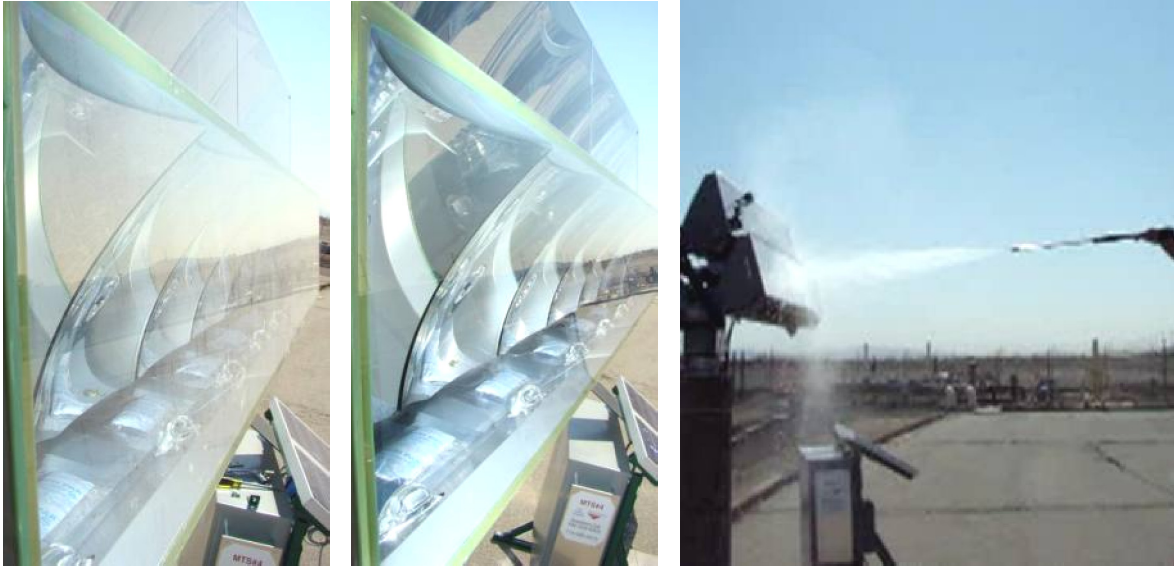
Fig. 16-a,b,c: Cover glass cleanliness before and after the 4 sec pressure spray wash shown.
