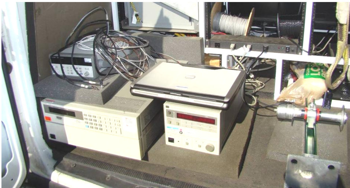
Fig. 6: Agilent IV Curve lab equipment supported by an AC inverter from the equipment van.
