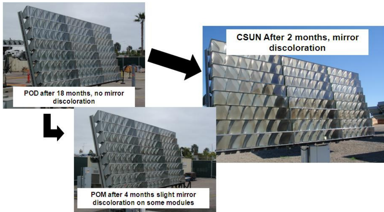
Figure 8-12. Seal Beach POD and POM panels and a CSUN power plant panel.
