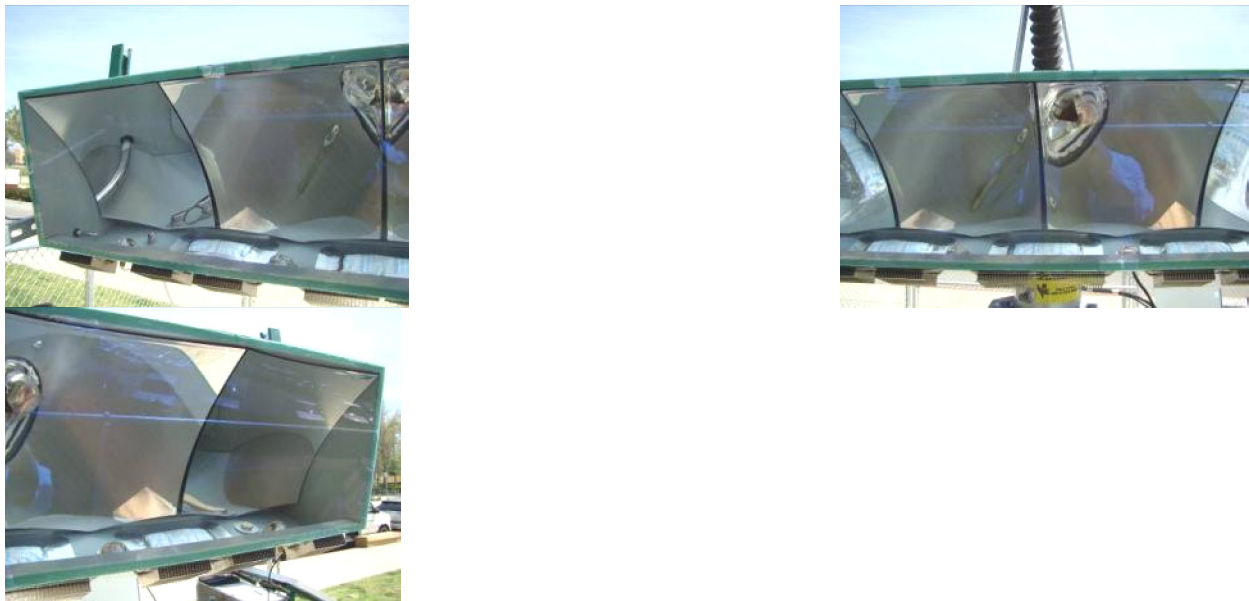
Fig. 12-a,b,c: Module mirror elements and chassis interior showing desiccant bags.
