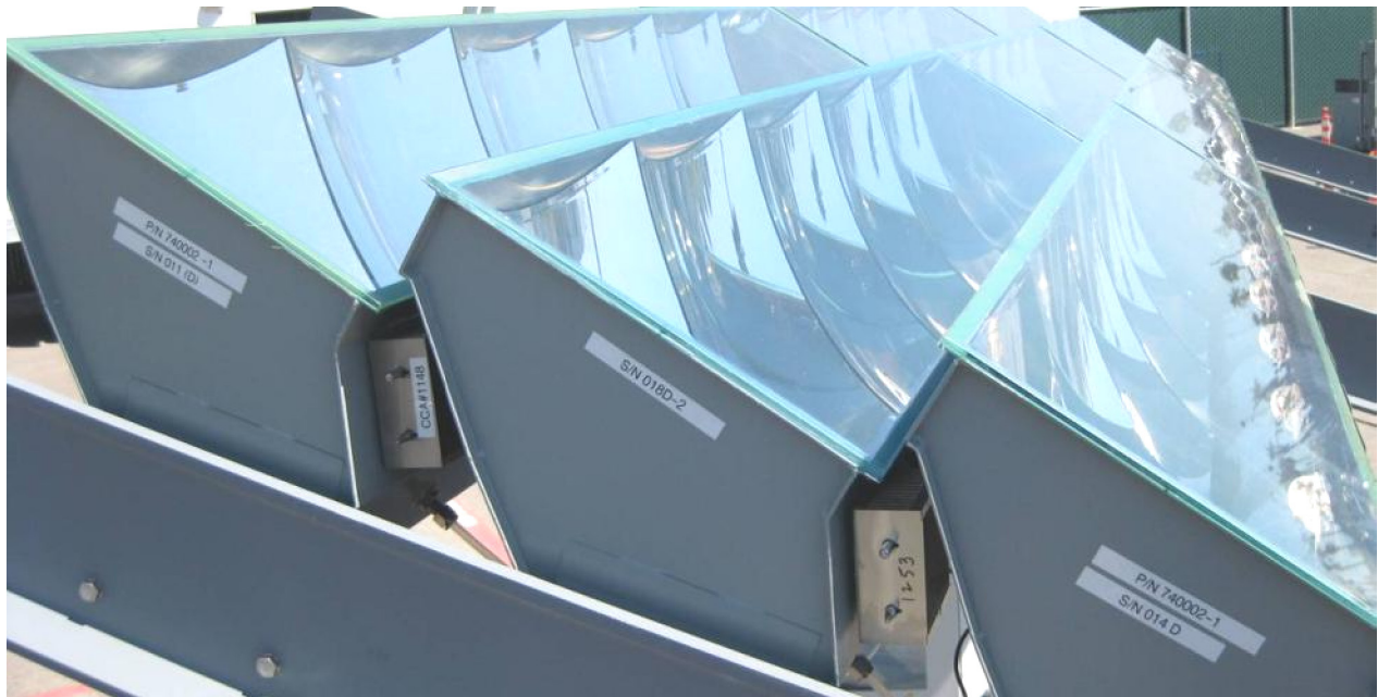
Fig. 1: POD Modules as they array together for a close packing factor.
