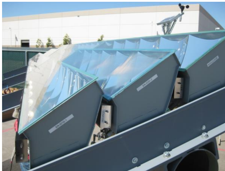
Figure 7-6. Modules mounted on the array tracker for testing.
