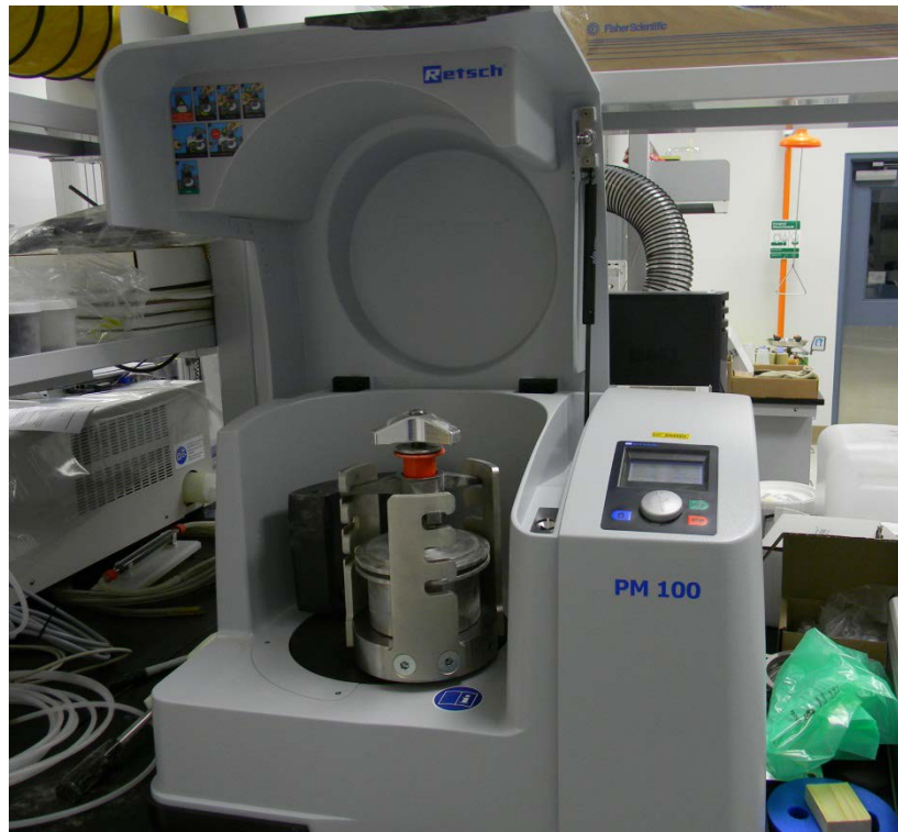
Figure 11. Laboratory ball mill for pre-treating Hg contaminated soils
