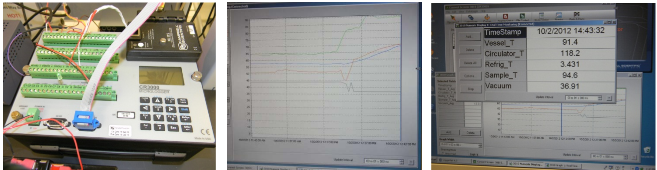
Figure 9. Data logger (left) and real-time display of temperature and pressure data
