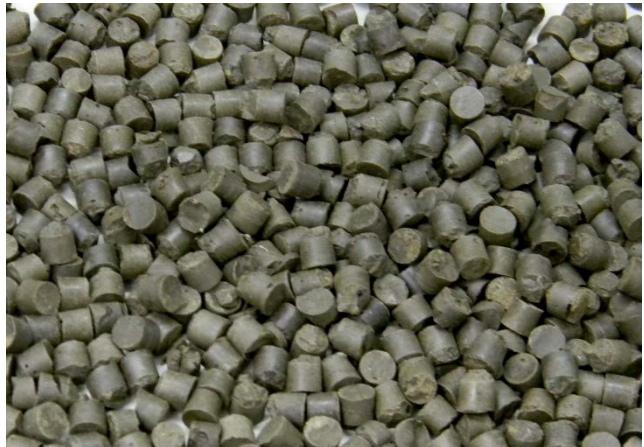
Figure 15 TCLP pellets being prepared (left) and ready for testing (right)
