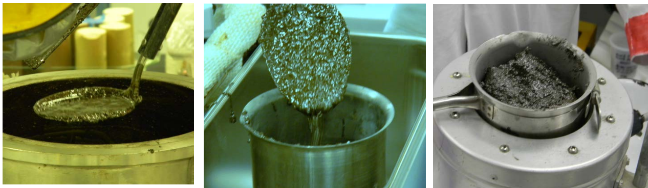
Figure 18. Comparison of melt viscosity for 40 (left), 50 (center) and 60 wt% (right) loadings
