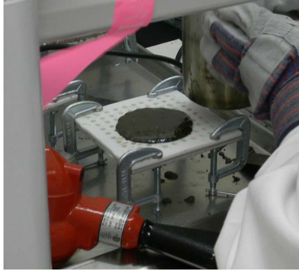
Figure 14 Preparing TCLP pellets by pouring into Teflon molds
