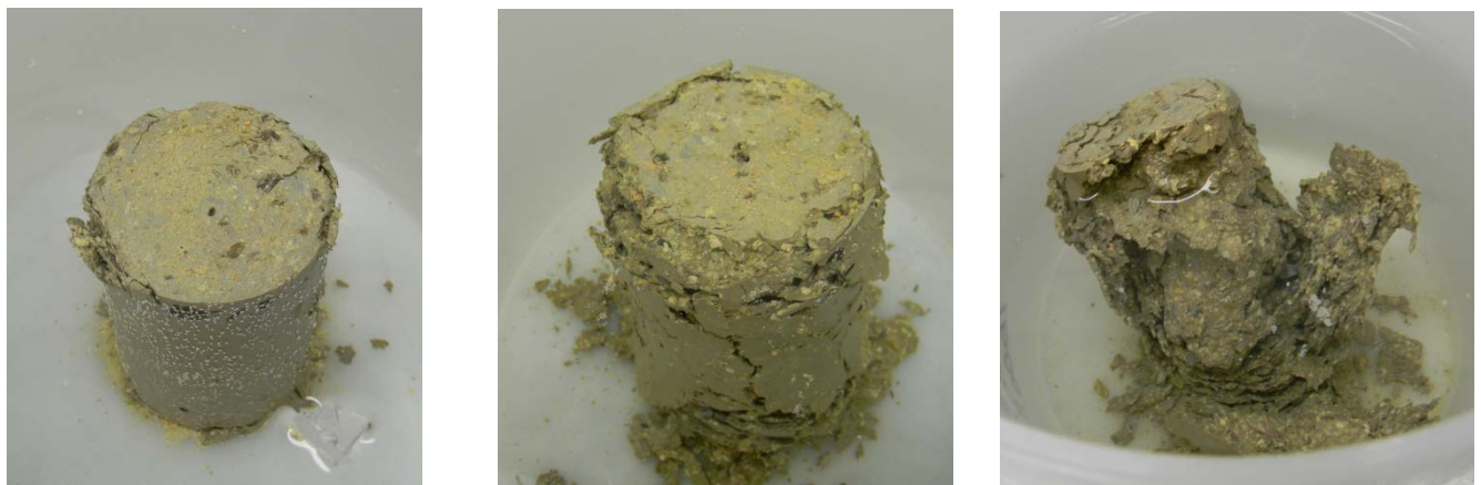
Figure 23. 50 wt% Y-12 Soil in Immersion after 18 hrs (left), 7 days (center), and 11 days (right)
