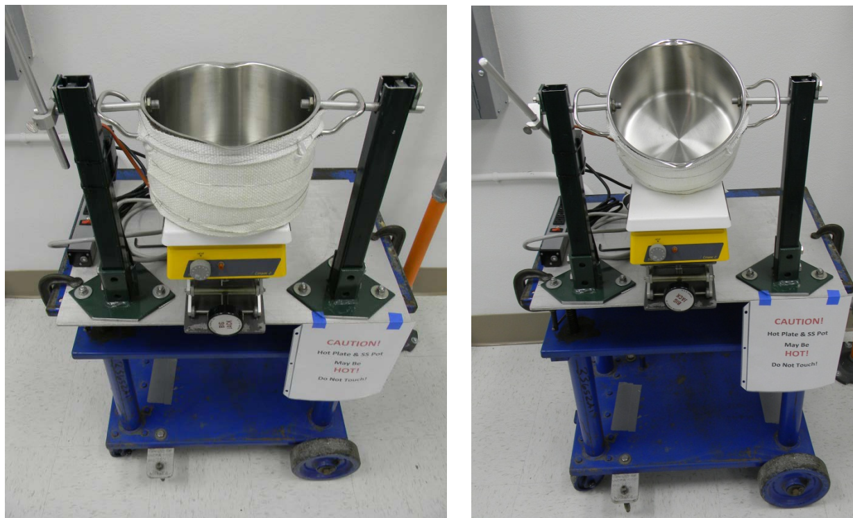
Figure 10. Heated vessel for pouring waste forms
