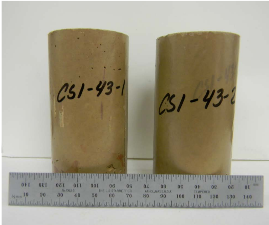
Figure 22. SPSS Treated 43 wt% Y-12 Soil Samples Following 65 days in Water Immersion
