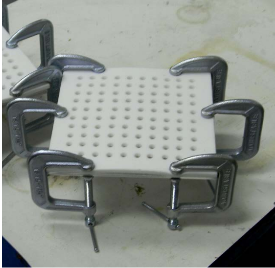
Figure 14 Preparing TCLP pellets by pouring into Teflon molds
