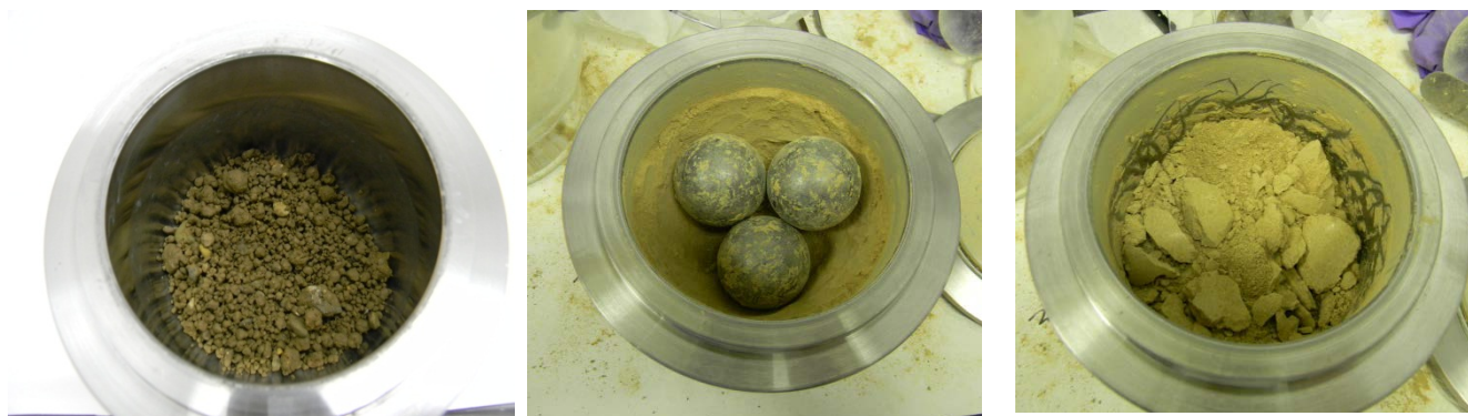
Figure 19. Ball mill pre-treatment of Y-12 soil before (left) and after (right) processing. Balls shown in center.
