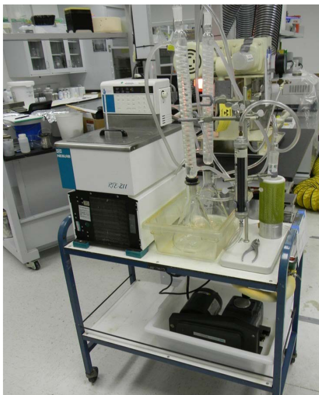
Figure 7. Off-gas treatment system (left) with close-up of condensate collection (right)
