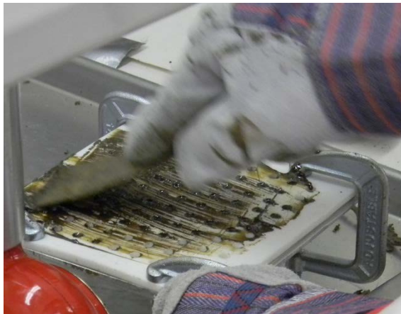
Figure 15 TCLP pellets being prepared (left) and ready for testing (right)
