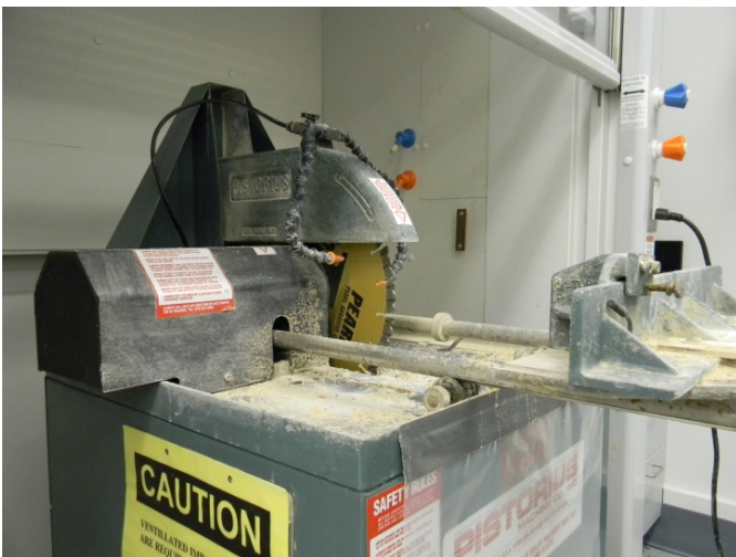
Figure 13. Diamond tipped wet saw (left) for cutting cylindrical test samples (right)
