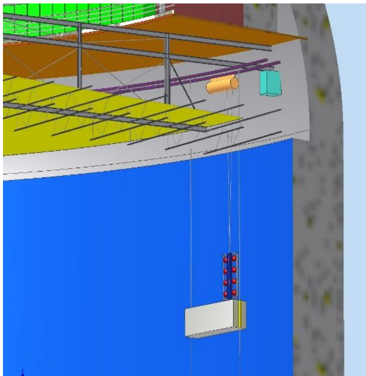
Figure 2-22: Gondola installing light shield and routing signal cables
