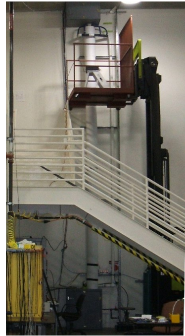
Figure 5–5: Photographs of external water transparency measurement devices at LLNL (horizontal) at left and UCI (vertical) at right.
