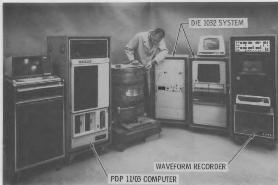
Figure 1. Acoustic Emission Detection/Analysis System
