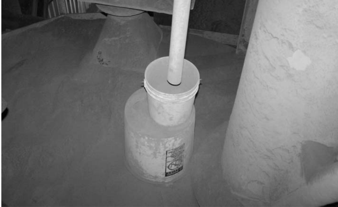
Figure 4-13: Portland Cement Sampling Point
