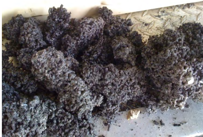
Figure 10-19: Poultry litter pellet clinkers from 40% pellet run
