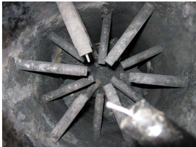
Figure 10-20: View from top of gasifier of poultry litter pellet clinkers hung up between levels 3 and 4 after loose biomass char had been removed. Level 5 is obscured by clinkers
