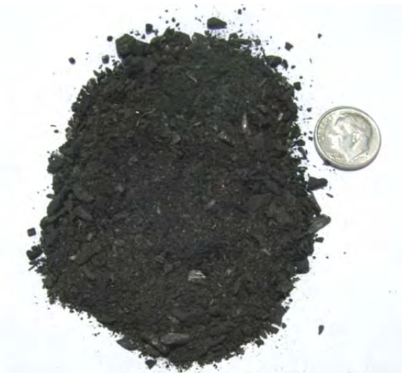
Figure 10-29: Char collected from chamber below gasifier grate, labeled 'Below Grate'
