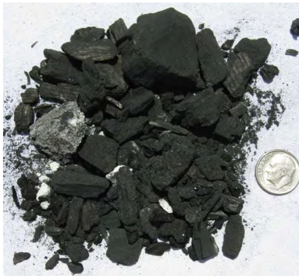
Figure 10-28: 'Rest of Gasifier' sample, comprised mostly of charcoal and wood char
