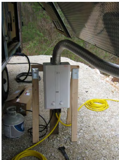
Figure 9-17: Propane water heater used for flue gas generation
