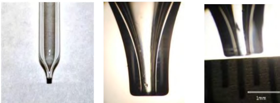
Figure 2-15: Glass nozzles for the piezoelectric drop generator
