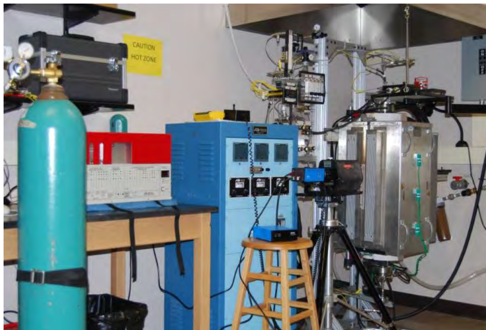
Figure 2-1: Photograph of the burn simulator system with visualization setup
