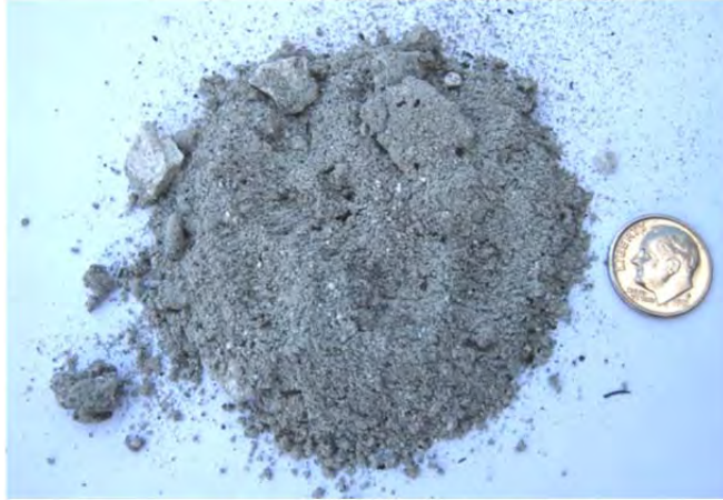
Figure 10-27: Crumbled poultry litter ash as sent for analysis in one experiment for each limestone set point (3.71, 5.71, and 7.71 % Lime/Wet PL), labeled 'PL Ash'
