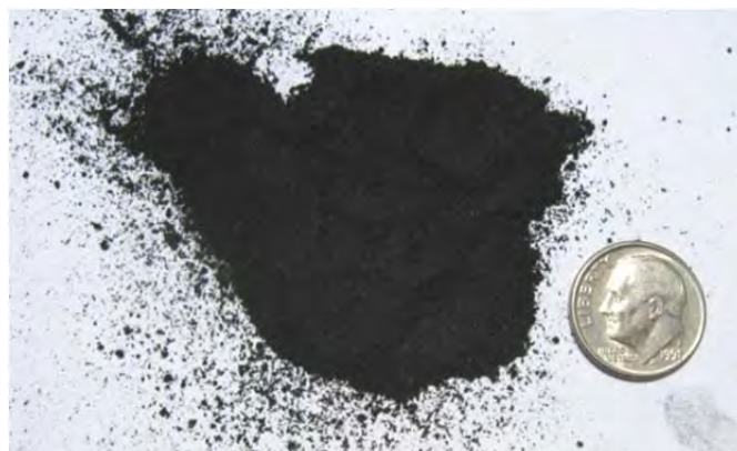
Figure 10-31: Char collected from filter box, labeled 'Filter'
