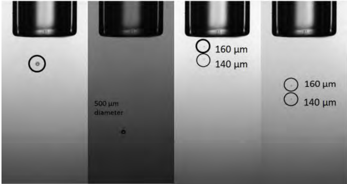
Figure 2-28: Images of 50 % glycerin droplets produced at 3.0 Hz, 0.01 \mu\text{L}/\text{min} , 55 V drive amplitude. Images are taken using PCO camera with Nikon 105mm lens at 143 FPS
