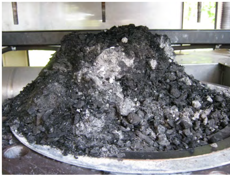
Figure 10-26: Ash mound as seen when gasifier is opened at crack above grate. Poultry litter ash is the light gray section in the middle of the mound
