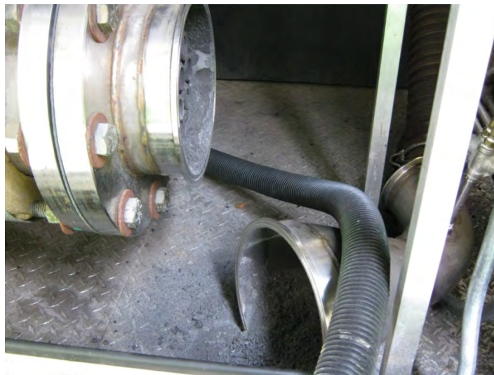
Figure 9-11: Heat exchanger exit, tubes visible inside at left. Pipe bend and flexible hose leading to filter box at right
