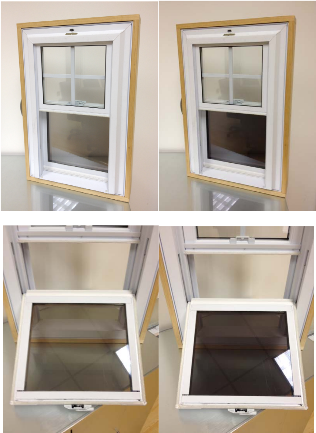
Figure 14. A demo window made with 1ft × 1ft ALCW film laminated to the glass surface of the bottom panel. The window is driven either with a small battery embedded in the window frame or with a small solar cell mounted on the top portion of the frame.
