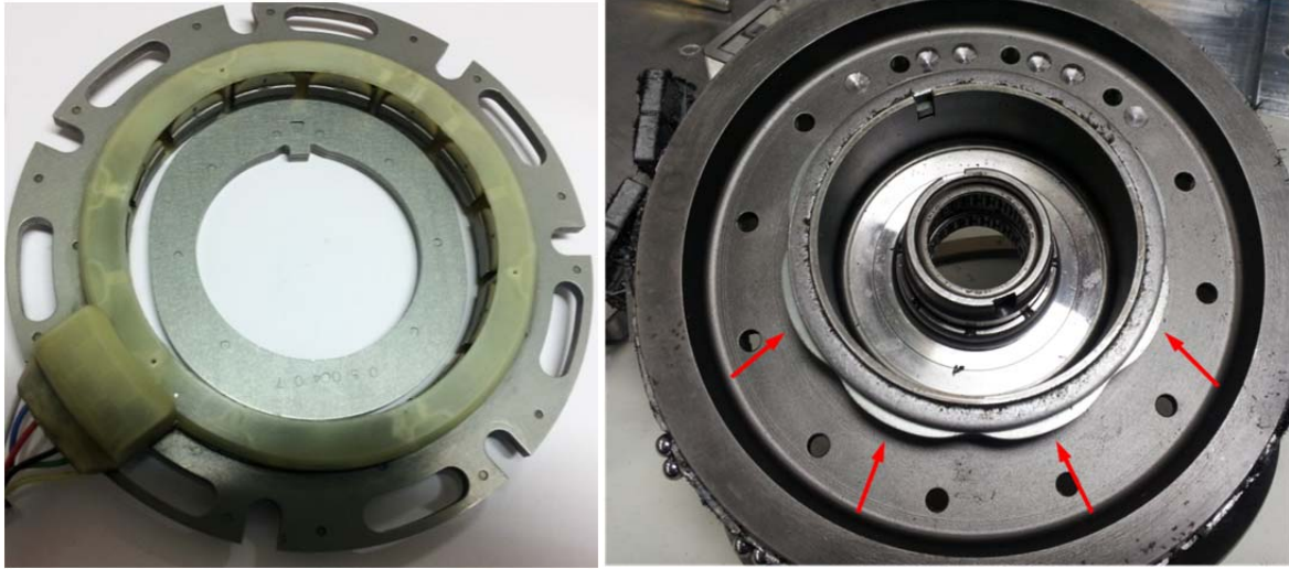
Fig. 53. Toyota Prius motor resolver (left) and Hyundai Sonata motor resolver (right).
