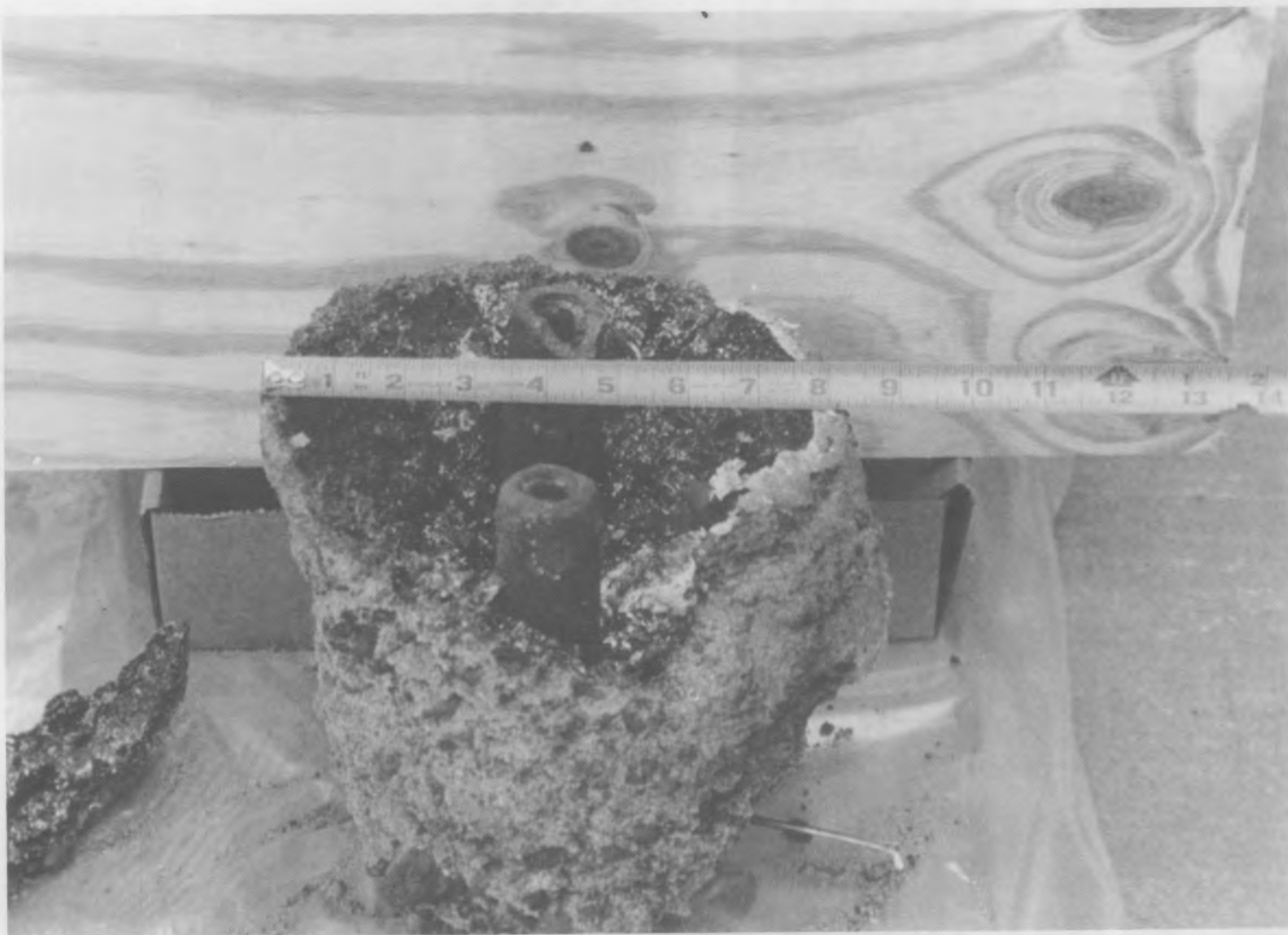
FIGURE 10. AEDC Site 1 Vitrified Block (8803810-17CN)
