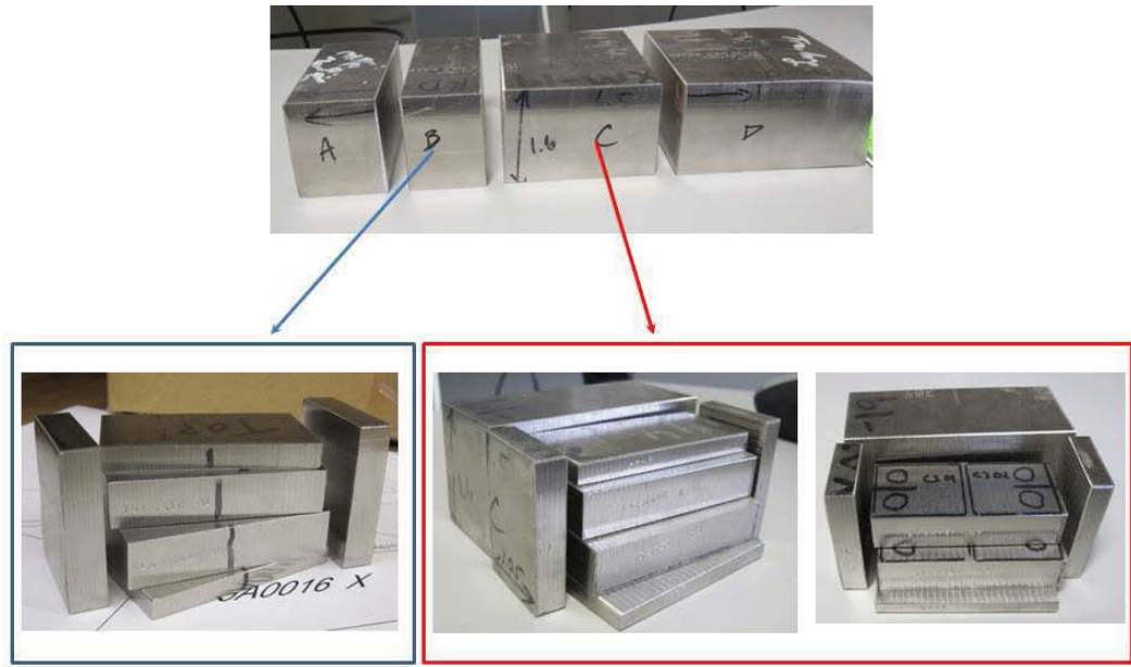
Figure B-4: Baseline SCC specimen extraction from 19.3% cold worked alloy XM-19
