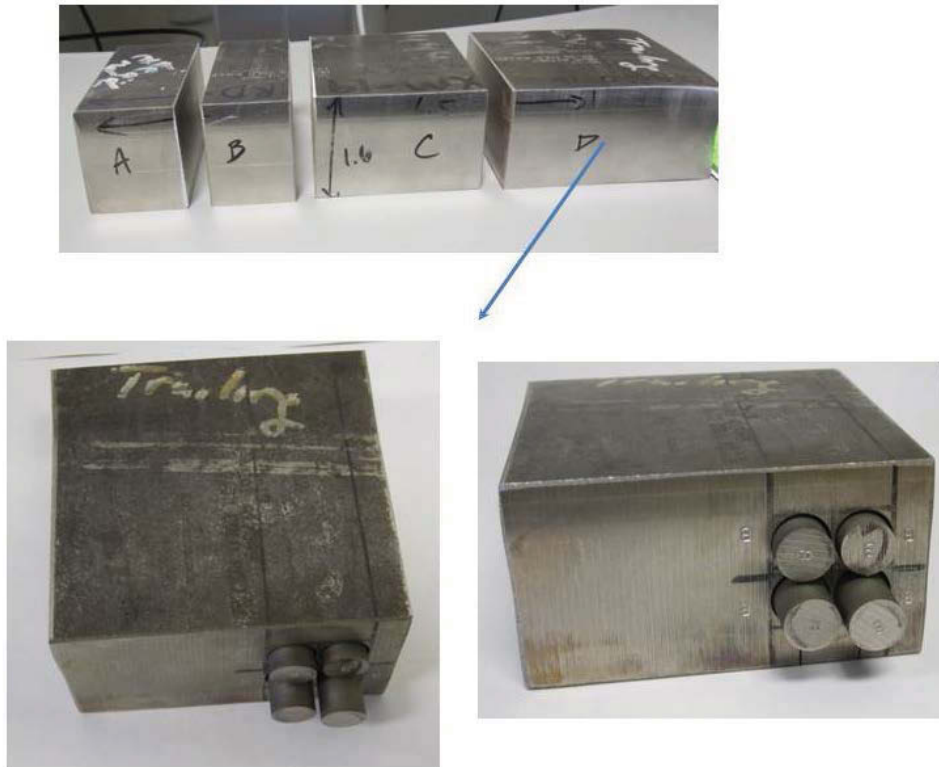
Figure B-6: Baseline tensile specimen extraction for 19.3% cold worked alloy XM-19
