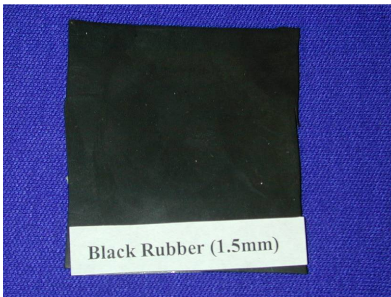
Figure A.12. Digital Photograph of the Thick Black Rubber Membrane Material Sample
