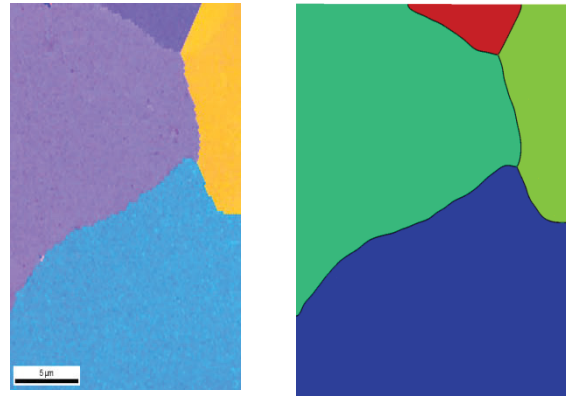
FIGURE 1. Microstructure reconstruction in MARMOT of a high burnup MOX fuel, where the EBSD scan is shown on the left and the reconstruction is shown on the right.
