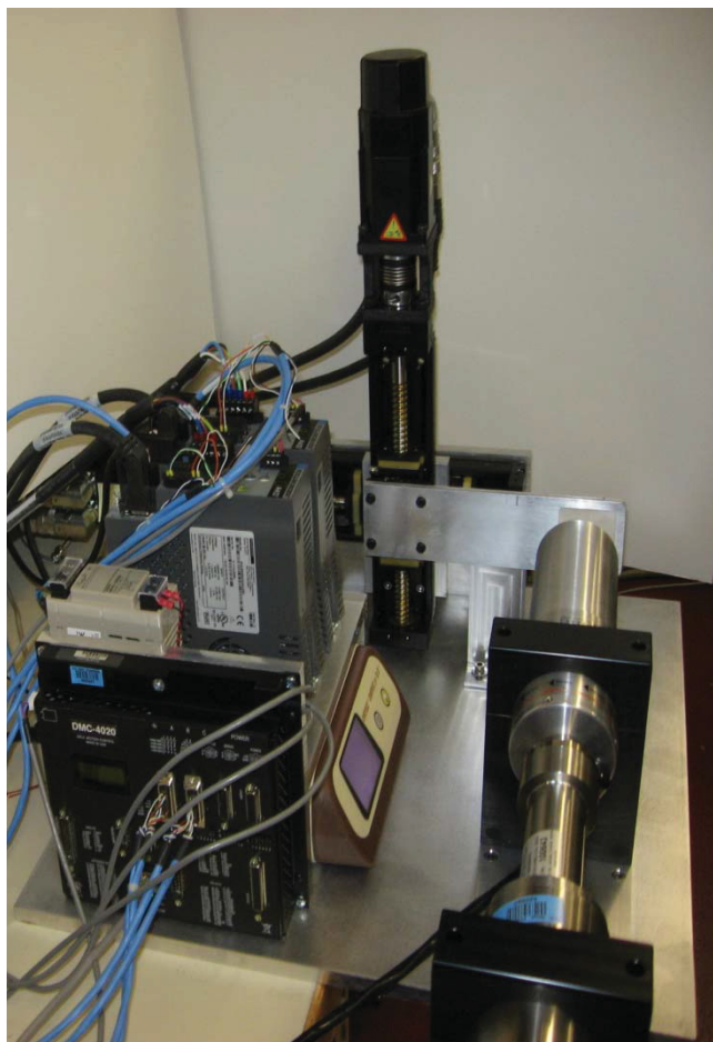
FIGURE 3. SRPA rad-hardened scan bed with two detectors.
