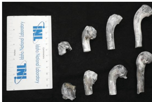
FIGURE 1. Residual projectiles that were captured after perforating targets.
