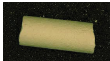
FIGURE 5. Portion of sintered CeO 2 rod originated from a Dry-Bag Isostatic Pressed, long “green” rod.
