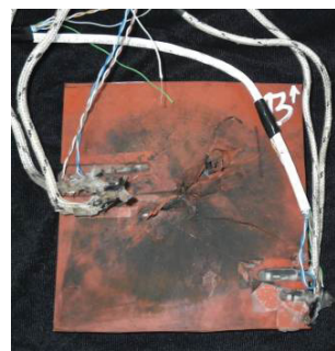
FIGURE 2. A polymer layer with embedded thermocouples to measure temperature during ballistic impact.
