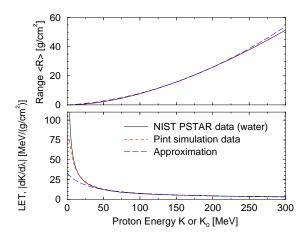
Fig. 1. Linear energy transfer  $|dK/d\lambda|$  and mean range  $\langle R \rangle$  for protons in water, versus local kinetic energy K or initial kinetic energy  $K_0$ . Data are shown for NIST PSTAR reference data, pint Monte Carlo simulation, and the approximations of Eqs. 1 and 3.
