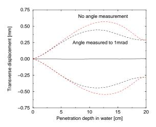
Fig. 4. A comparison of most likely paths and  $1\sigma$  RMS envelopes, simulated for 200 MeV protons by pint Monte Carlo, with no knowledge of the exit proton angle and with exit proton angle known to 1 mrad. Exit angle constraints improve the most likely path uncertainty by up to 40%.
