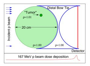
Fig. 5. Schematic layout of object being radiographed, plus compensating 'Bow tie'. The simple phantom shown at the bottom has been used in preliminary reconstruction simulations. [4]
