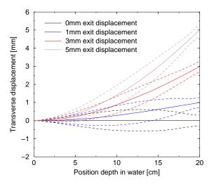
Fig. 3. Illustration of most likely paths and  $1\sigma$  RMS envelopes, simulated for 200 MeV protons by pint Monte Carlo. The entrance position and angle are assumed known to sub-mm accuracy, and the exit displacement is assumed known to a 1 mm detector resolution.
