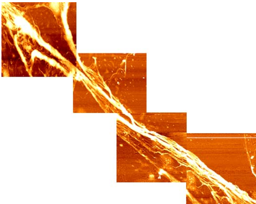
Figure 17: A series of consecutive AFM images taken from the same region of a coated slide showing long bundles of AuNW. Each square is 20 \mu\text{m} x 20 \mu\text{m} .
