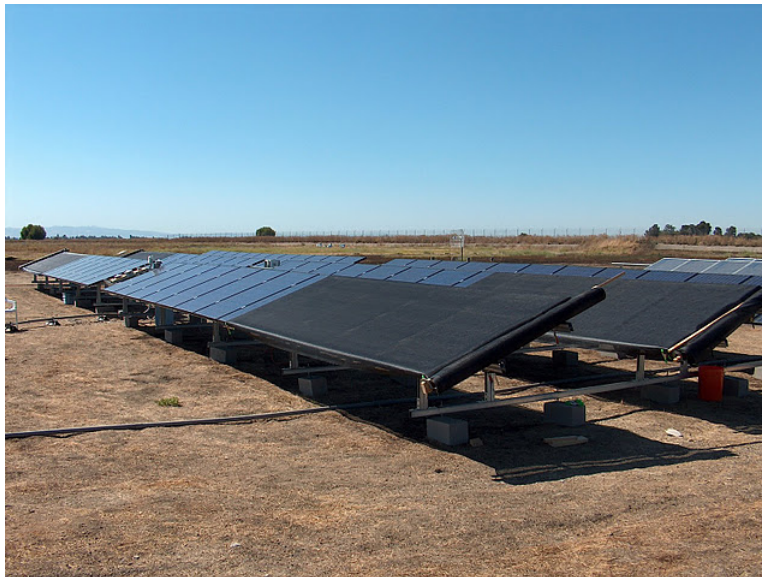
Figure 12. Image showing the two arrays at the test yard in Davis, California. The reference array is on the right, and the Enphase array is on the left. Both arrays are shaded in the (14:14:0) configuration. The irradiance sensors and met station are centrally located in the front row between the two arrays.
