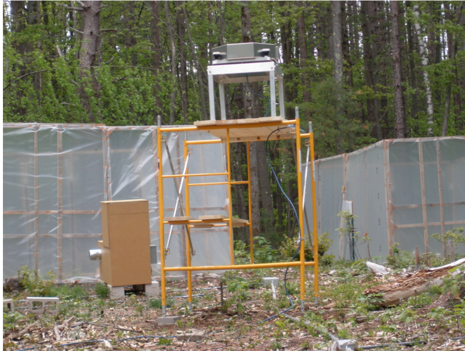
Figure 2. May 2009 Remtech PA1 sodar installation at the Ant and Climate Change experiment.
