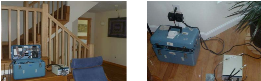
Figure 57. Active samplers for PFT (blue box) and VOC and aldehydes (peristaltic pump)
