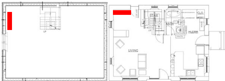
Figure 3. Floor plans and position of the mini-split indoor units (red boxes) in the Stow home Left: Basement. Right: 1st floor. The positions of the mini-split indoor units are marked by the red boxes.
