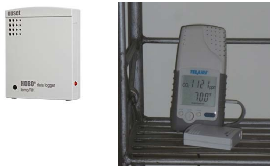
Figure 8. Left: Loggers used for temporary indoor measurements. Right: The loggers have external channels for additional sensors; e.g., for CO 2 concentration.
