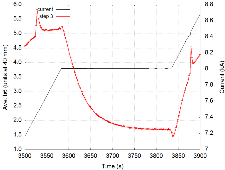
Figure 45 Decay of b_6 during the 8 kA holding (step 3, 250 mm probe).
