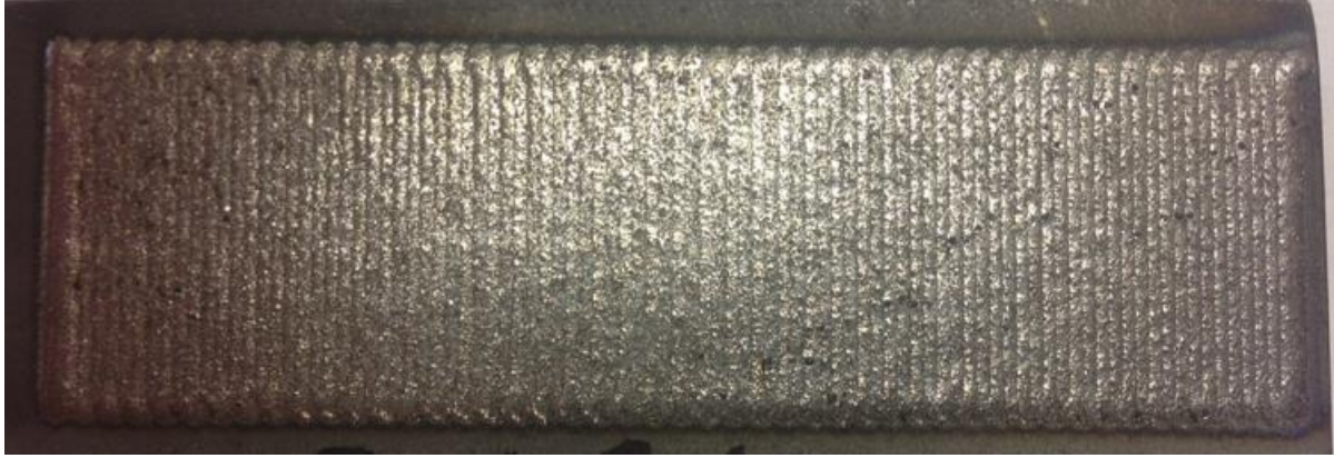
Figure 26: Alloy 1 fused coating fabricated using the POM laser deposition system.
