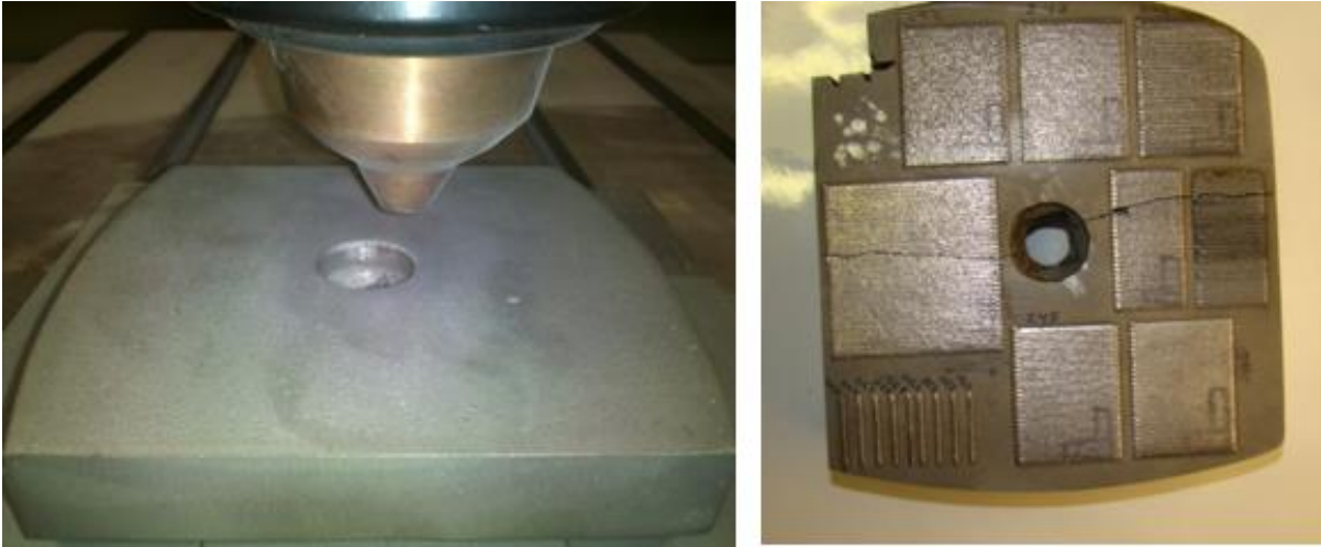
Figure 54. Laser fusing setup of the mixing paddle in the POM laser (left). Various laser fusing trials for 7 powders on paddle.
