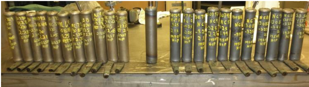
Figure 38: HIP samples from Alloy 1-10 at 1950F and 2125F.
