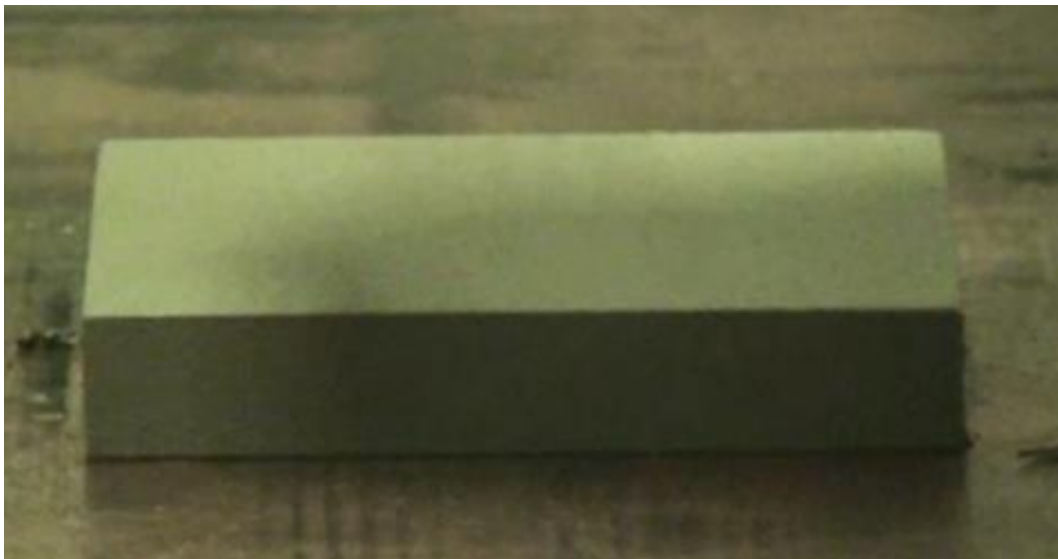
Figure 19: Coated coupon utilized in laser fusing with the 4 kW Nd:YAG laser system.
