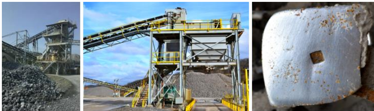
Figure 53. Vulcan Materials Dixie Lee Rock Quarry (left), fine aggregate rock mixing machine (center), and a worn mixing paddle (right).
