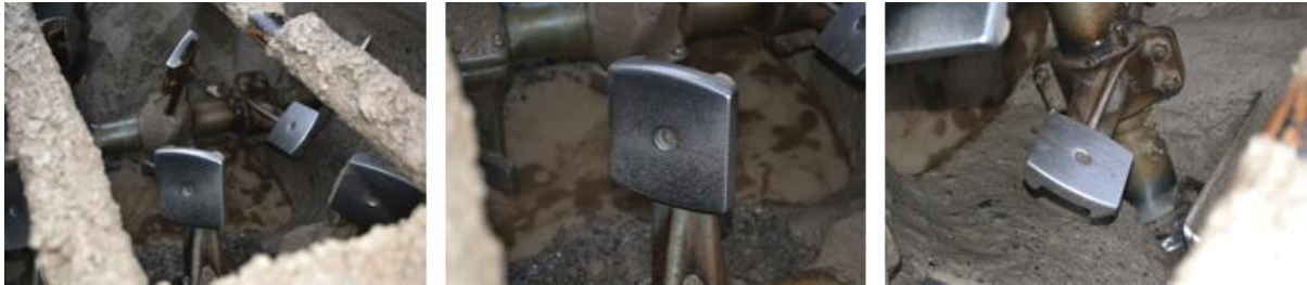
Figure 57. Annual inspection of paddles (left). The nanocomposite coatings were still intact and appeared to be in good shape (center). The uncoated paddle installed at the same time exhibited visual signs of light abrasion, but were in good condition (right).
