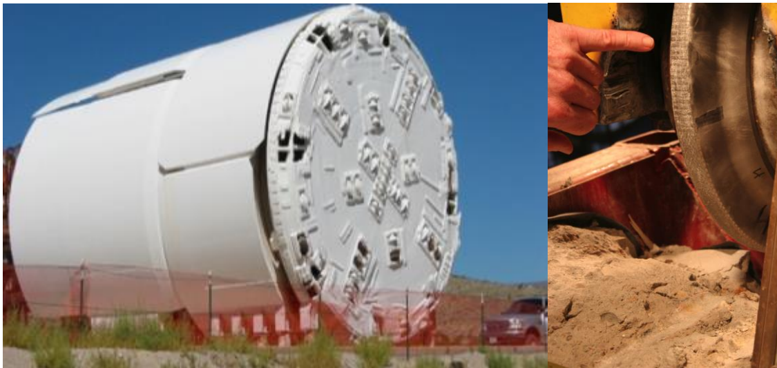
Figure 2. Tunnel boring machine used to construct the tunnel at Yucca Mountain (Left). Nanocomposite Coatings Tested on Disc Cutter at the Colorado School of Mines Linear Cutting Machine (Right).
