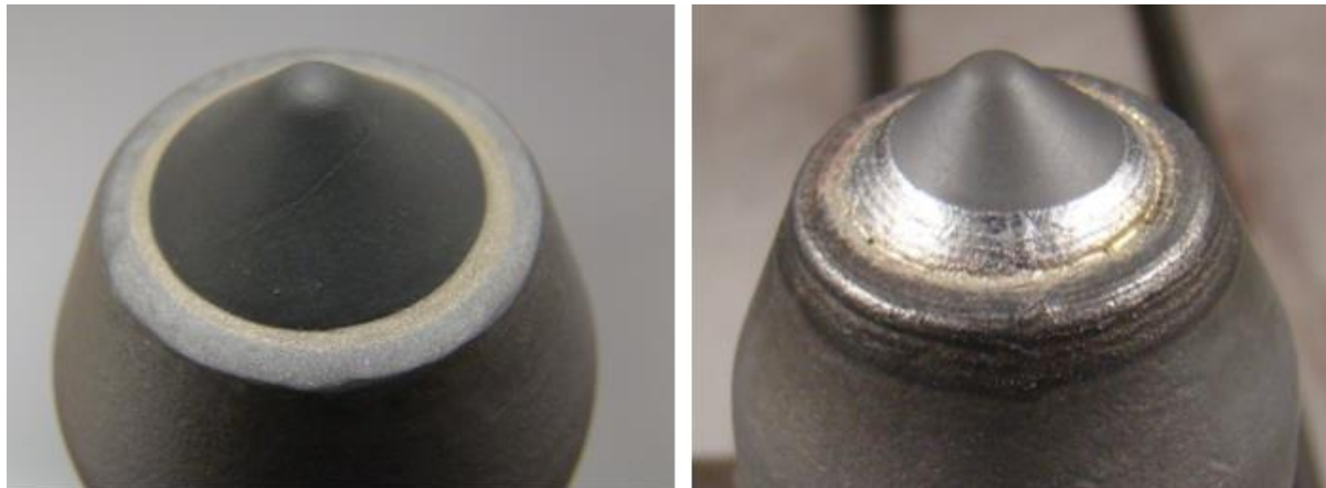
Figure 60. Conical Tool before and after laser coating with Alloy 8. Coating of the shoulder of the conical tool results in increased wear performance and maintains the integrity of the WC/Co insert. The coating did not effect or crack the insert during the deposition process.
