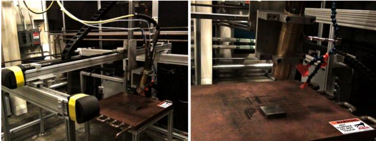
Figure 20: 4 kW Nd:YAG laser system utilized to fuse coatings onto coupons. The gantry system for the laser is computer controlled.
