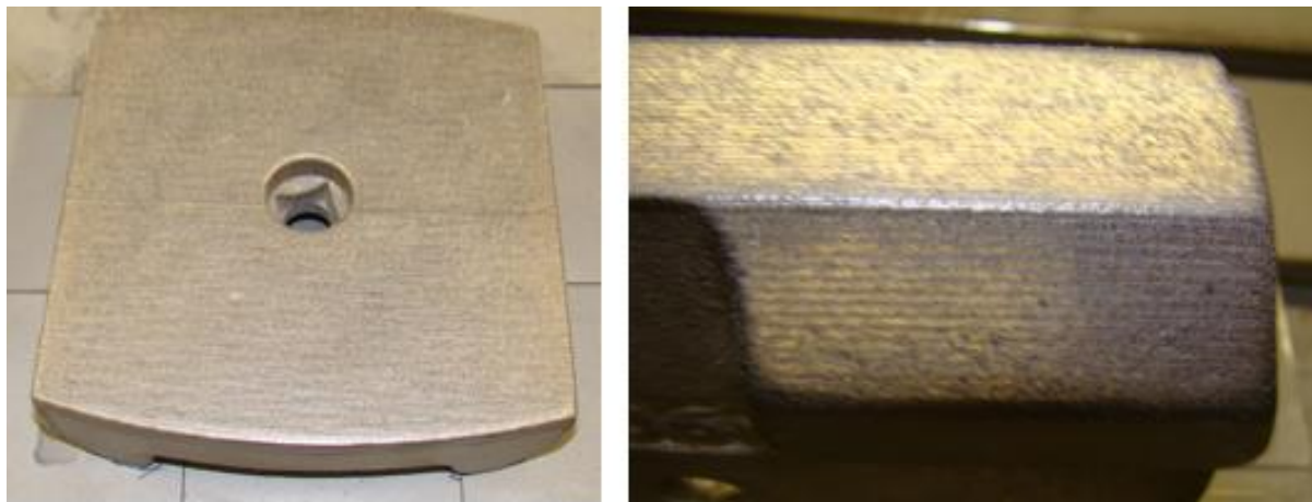
Figure 56. Laser fused nanocomposite coating on mixing paddles showing front face (left) and sides (right).
