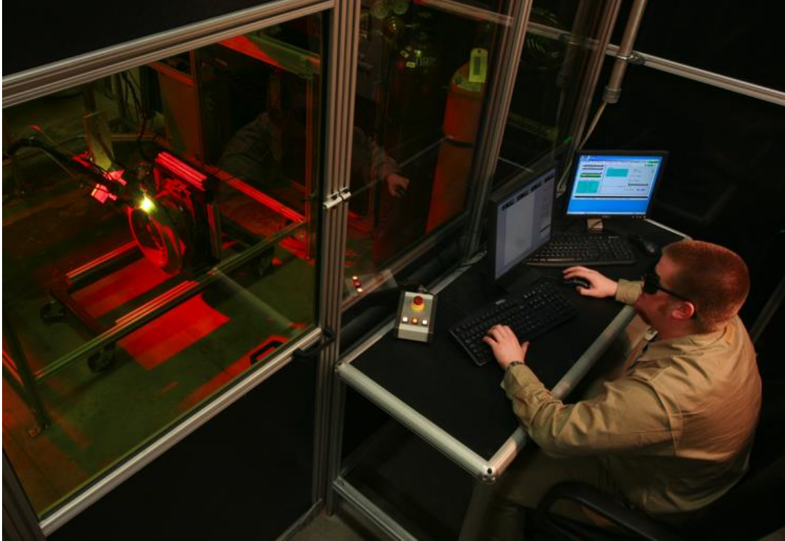
Figure 5. Original laser processing setup for applying laser coatings to disc cutters.
