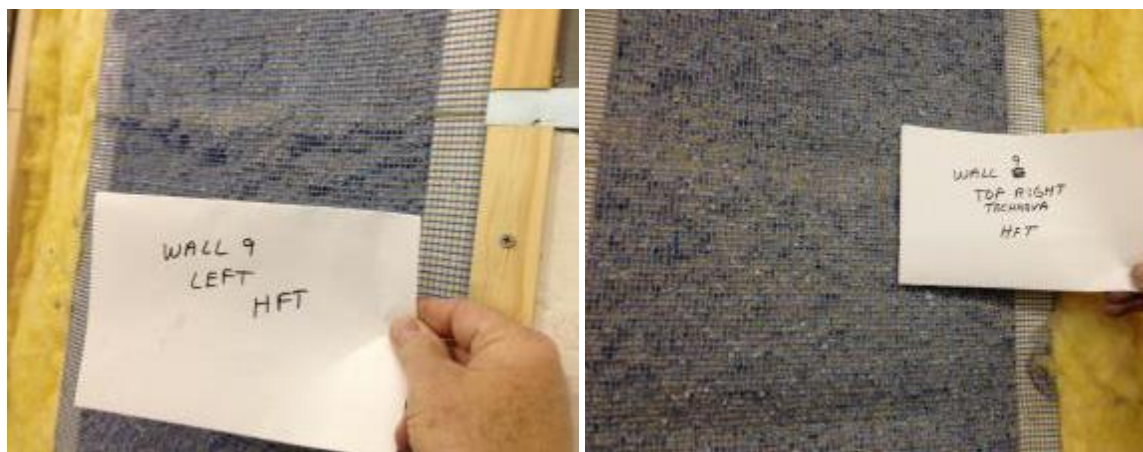
Figure 12. Gypsum (left) and ‘Dispersed Nano-PCM’ (right) sections from ‘Test wall 2’; the gypsum section exhibited air gaps near the sensors.
