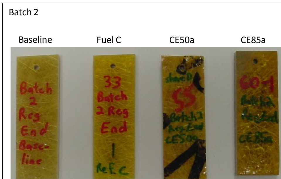
Fig. 13. Photograph showing the Batch 2 specimens before and after exposure to Fuel C, CE50a, and CE85a.
