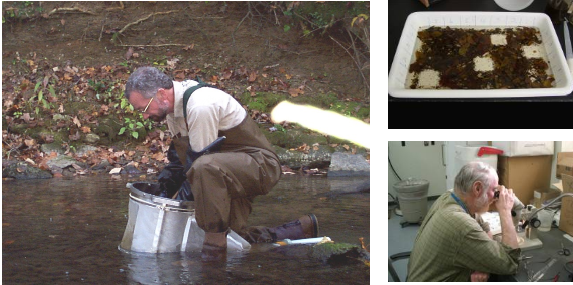
Fig. 5. Benthic macroinvertebrate community task sampling using a Hess sampler (left), TDEC protocol laboratory sorting (top right), and taxa identification (bottom right).
