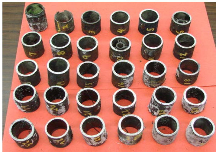
Fig. 35. Photo of the 30 samples removed from one of the corrosion probes. Samples #6 and #10 still contain the spacers used to position the support rod in the center of the probe. Several other samples still contain the remnants of the thermocouple that was attached to the outer surface of most samples.
