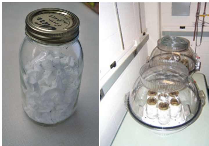
Figure 2. LiCl-KCl eutectic salt received from Idaho National Laboratory which was crushed and stored in mason jars (left) and stored inside desiccators (right) to prevent contact with air.
