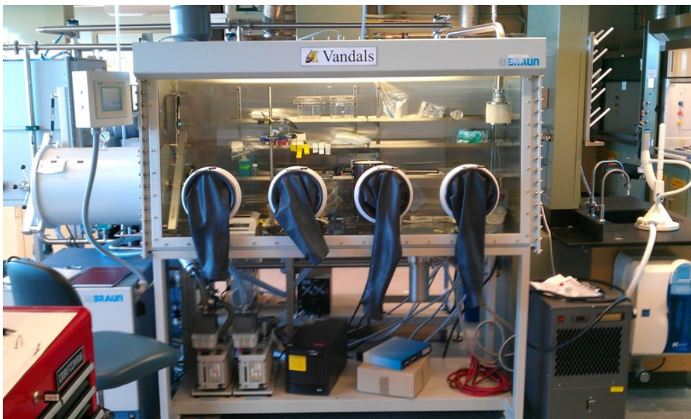
Figure 14. Radioactive material glove box used for depleted uranium electrochemistry work at INL.
