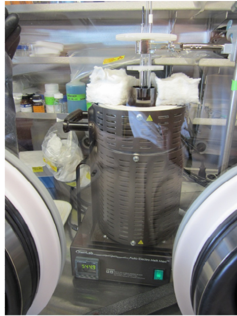
Figure 17. Thermcraft heater raised into position around the heater well (left). KerrLab Auto Electro Melt Maxi furnace positioned inside the glovebox (right).
