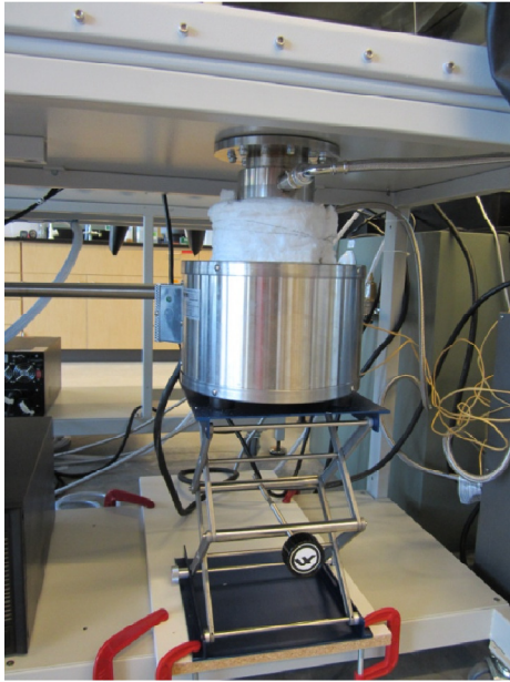
Figure 17. Thermcraft heater raised into position around the heater well (left). KerrLab Auto Electro Melt Maxi furnace positioned inside the glovebox (right).
