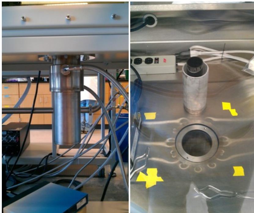
Figure 16. Heater well viewed from outside (left) and inside (right) of the glove box.
