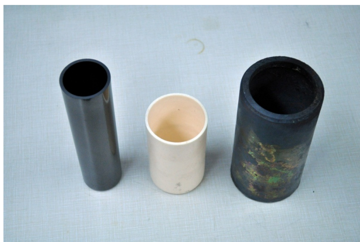
Figure 7. Glassy carbon (left), alumina (center), and stainless steel (right) crucibles used in the electrochemical cell.
