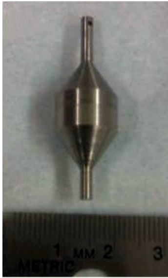
Figure 21. Nickel bob used to measure the density of the molten salt.
