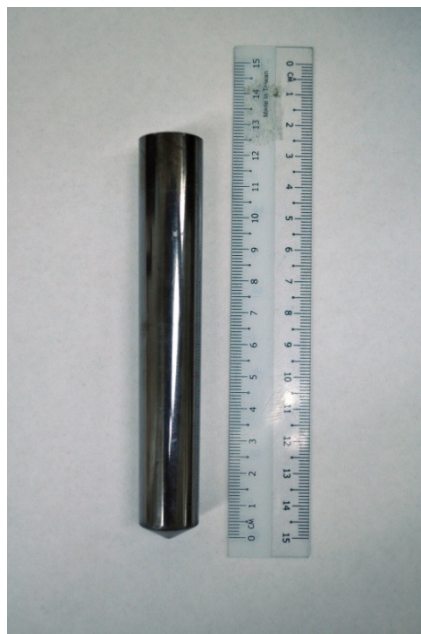
Figure 25. Glassy carbon crucibles used to melt DSC samples.
