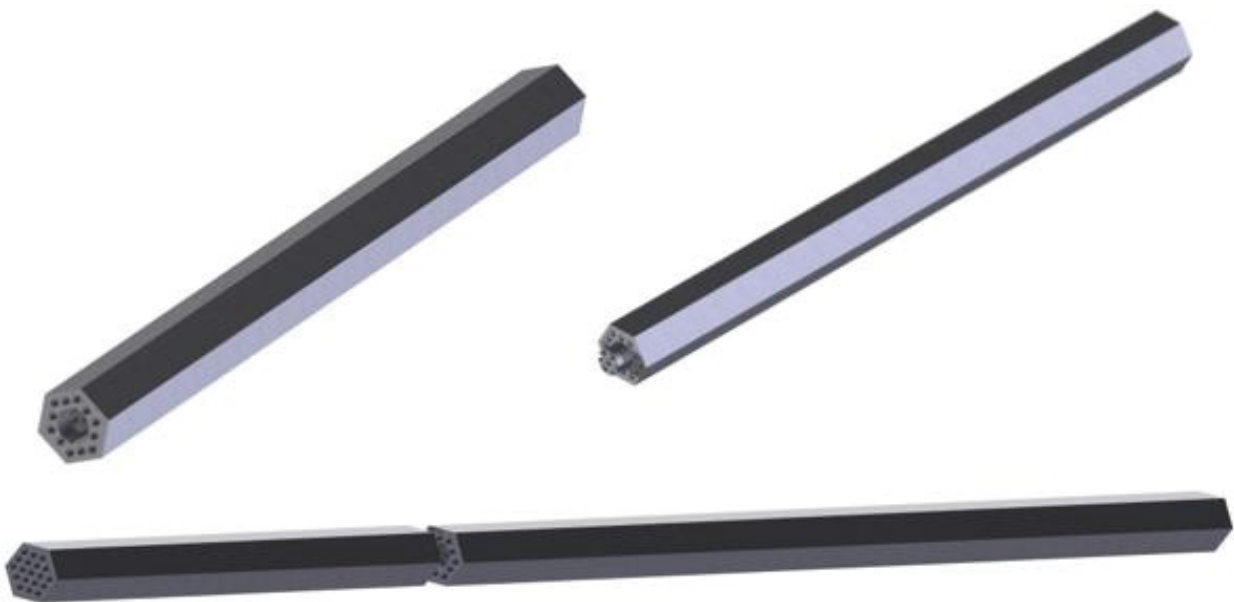
Figure 6: Assembly of cermet fuel elements from sections. Here, a fuel element with a 19-hole propellant flow channel configuration is assembled from 3 sections with end features that are keyed together.
