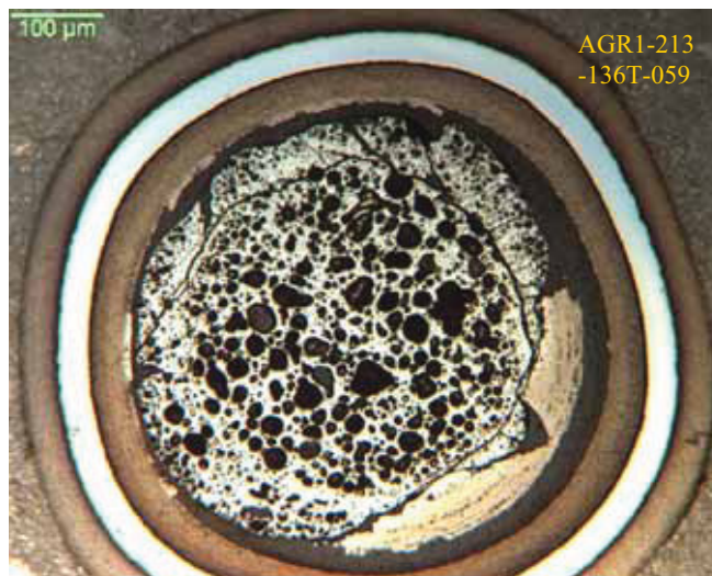
Figure 30. Extensive kernel swelling at a plane between separated pieces of buffer.
