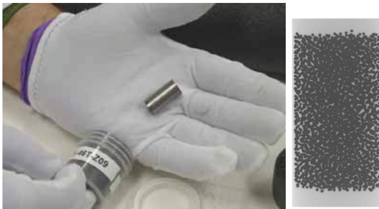
Figure 1. Photograph (left) and x-radiograph (right) of an unirradiated AGR-1 fuel compact.
