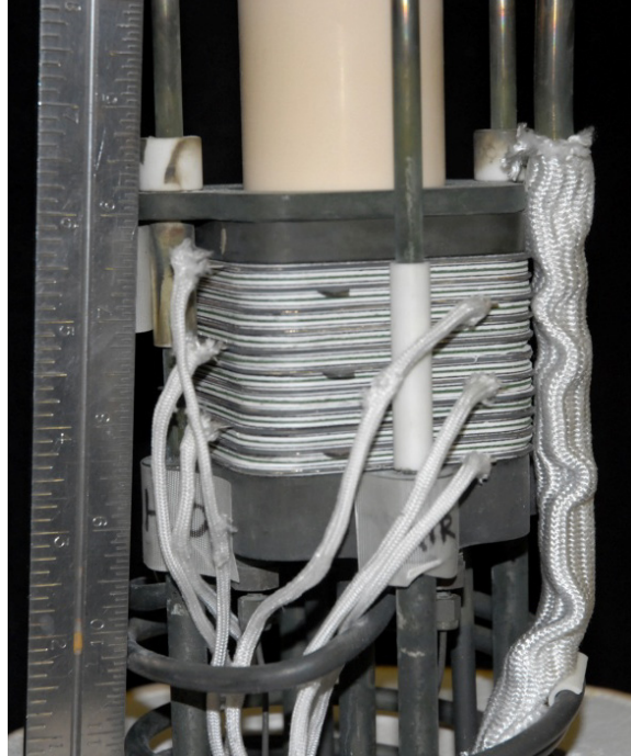
Figure 6. Installed 10-cell stack with intermediate voltage taps.
