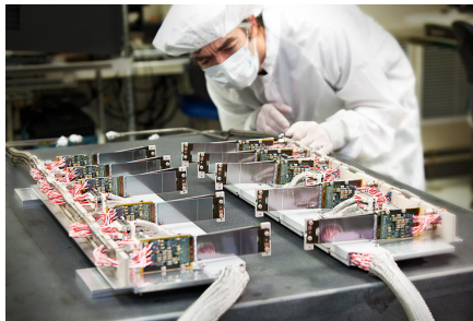
Figure 3: The two tracker halves of the HPS test tracker before integration.
