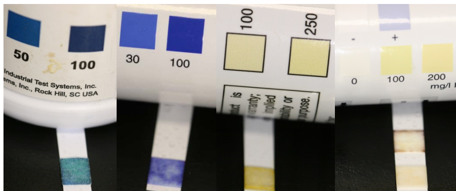
Figure 20 Test strips (24-27) of B with a peroxide concentration of 100 ppm.
