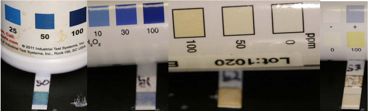
Figure 35 Test strips (50-53) of D (B normalized) with a peroxide concentration of 50 ppm.
