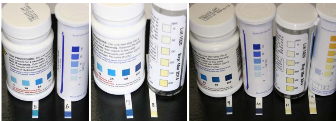
Figure 4 WaterWorks™ (5) and MQuant™ 1.10081.0001 (6) at 10 ppm (left), WaterWorks™ (7) and XploSens PS (8) at 50 ppm (middle), and WaterWorks™ (9), MQuant™ 1.10081.0001 (10), XploSens PS (11) at 100 ppm, and MQuant™ 1.10337.0001 at 100 ppm (right).
