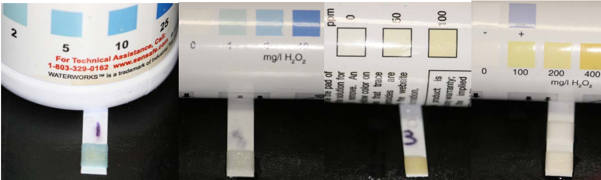
Figure 12 Test strips (1-4) of A with a peroxide concentration of 10 ppm.
