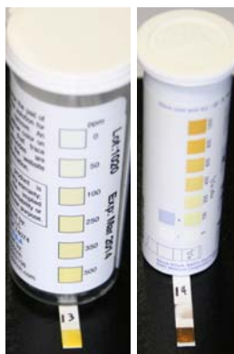
Figure 5 XploSens PS at 499 ppm (left) and MQuant™ 1.10337.0001 at 997 ppm (right).
