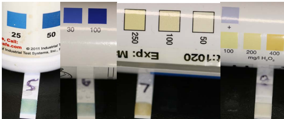
Figure 13 Test strips (5-8) of A with a peroxide concentration of 50 ppm.
