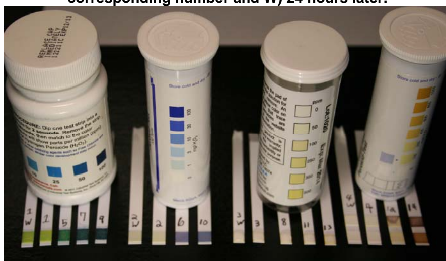
Figure 10 Peroxide test strips with additional blanks immersed in water (labeled with corresponding number and W) 96 hours after immersion in water.
