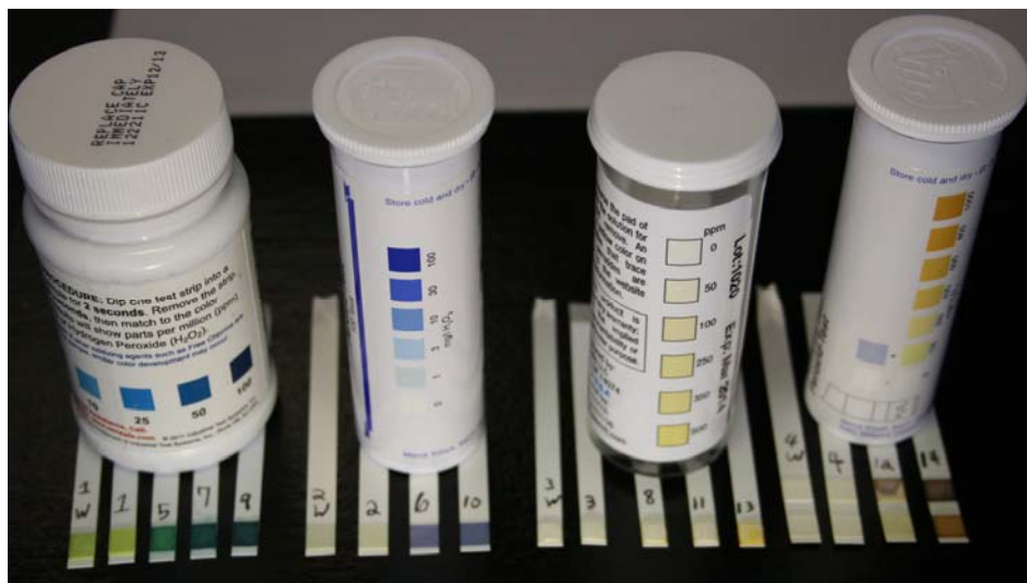
Figure 9 Peroxide test strips with additional blanks immersed in water (labeled with corresponding number and W) 24 hours later.
