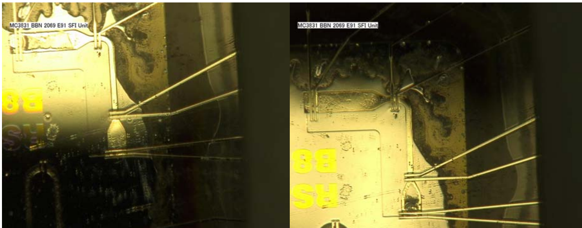
FIGURE 12: (1) Channel mostly filled with mercury. Film persists along all sides of channel not filled with bulk mercury. (2) Repeatability of mercury movement is attained.
