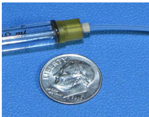
FIGURE 6: Specially modified syringe tip allowing for direct connection to desired tubing.
