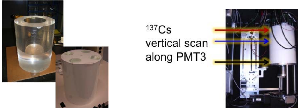
Figure 9. Left: Anticoincidence inner veto made of Ej200 Plastic Scintillator, wrapped in GORE diffuse reflector. Four low background R6041 Hamamatsu PMTs read scintillation light from the top. Right: Experimental set-up for source scans along the veto vertical side, in order to determine light collection uniformity and threshold.
