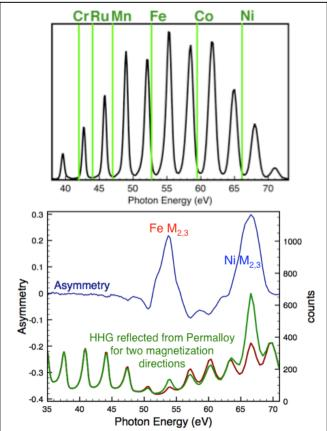
Fig. 2. (top) Experimental high harmonic emission (HHG) (black line) in the 40-70 eV photon energy region spanning the M absorption edges of several magnetic materials (green lines). (bottom) HHG spectrum reflected from the sample at an angle of 45 deg, for two different magnetization directions. The strong magnetic asymmetry signal for the Fe and Ni M-edges is also plotted. The asymmetry signal spans a few eV.
