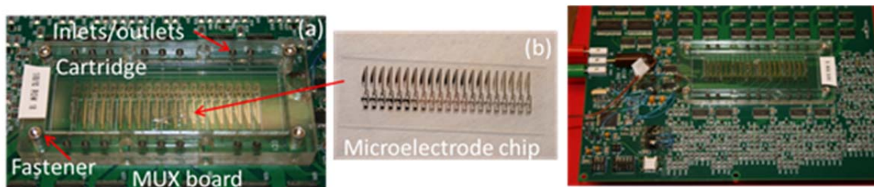
Figure 2. The new microelectrode slide chip also aligns to a previously developed MUX
