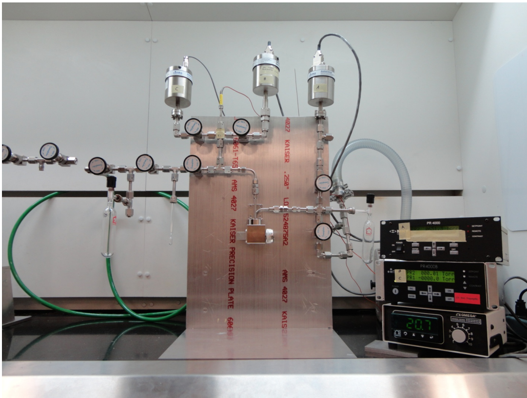
Figure 1. Photograph of the gas manifold setup.
