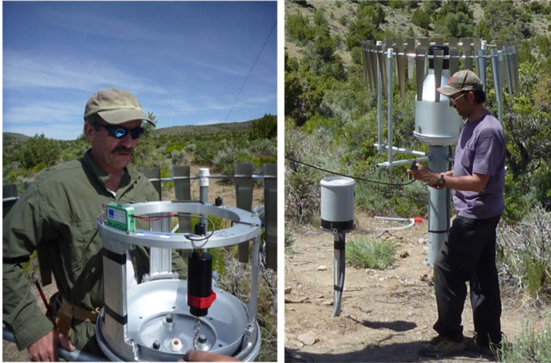
Figure 3. Geonor™ weighing precipitation gauge. The outer cover is removed in the left photo, with a view of the completed installation on the right. The secondary, tipping-bucket gauge can be seen to the left of the Geonor gauge.
