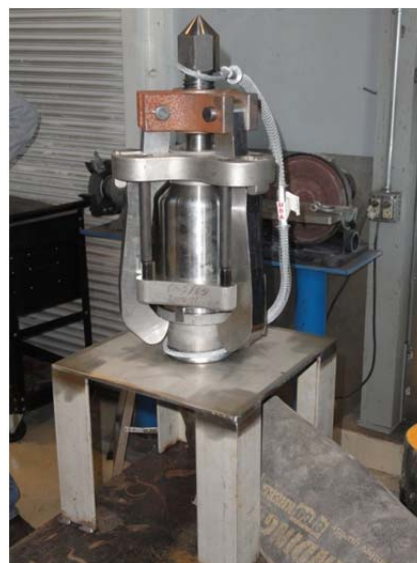
Connector test assembly (nozzle bottom is fitted with test port)
