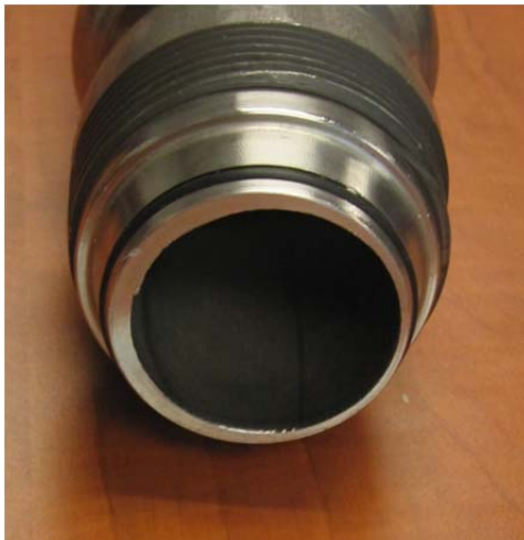
Figure 4. EPDM O-Ring on HIHTL End Fitting.
