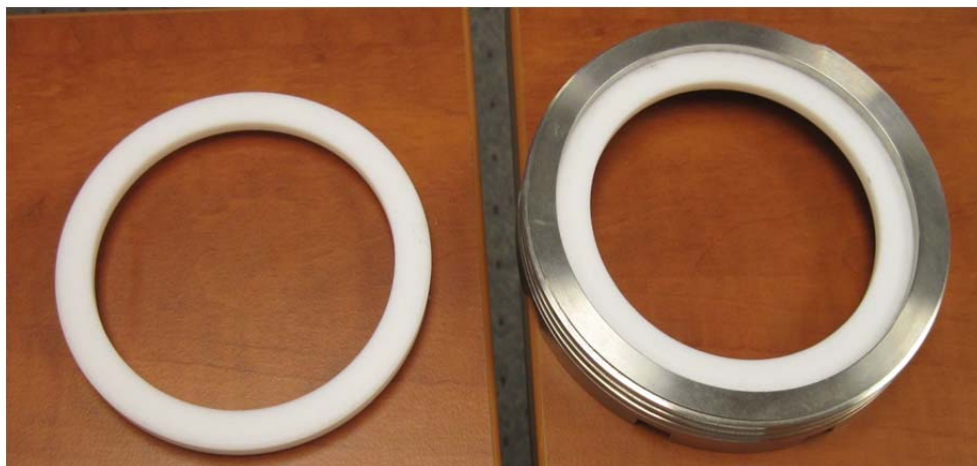
Figure 5. Teflon Gasket in Retaining Ring and Unconfined.
