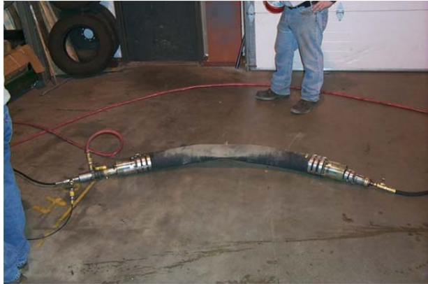
Hydro-testing of HIHTL coupons after crush test
