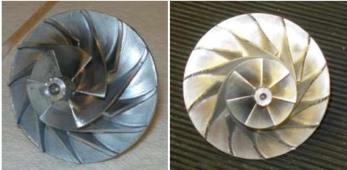
Figure 2-3. Main compressor (left) and recompressor (right) wheels.
